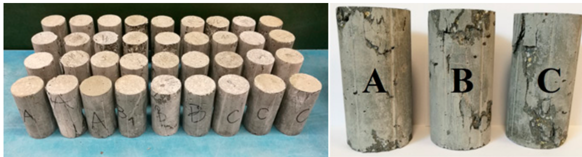
Figure 11. All of the samples after compression tests and the typical failure modes for tested concretes A, B, and C.
