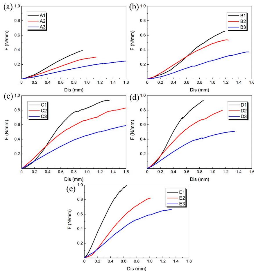
**Figure 7.** Radial force (per unit length) versus radial displacement curves for different groups of 3D-printed PLA vascular stents: from (a–e) are A, B, C, D and E group respectively.
