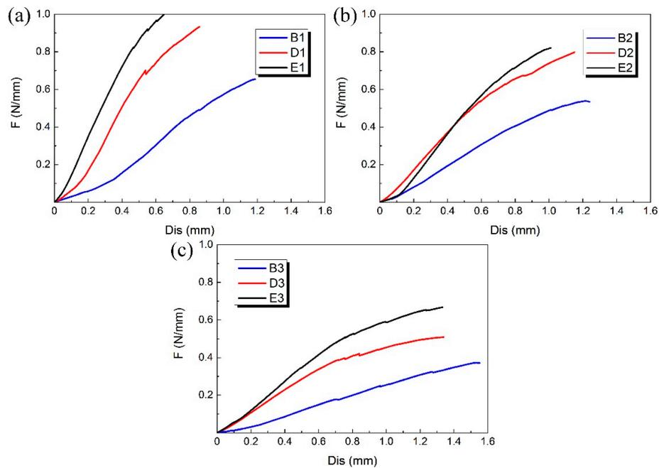
**Figure 9.** Radial force (per unit length) versus radial displacement curves for different geometric parameters of arrowhead NPR structure of 3D-printed PLA vascular stents: (a) PLA vascular stents with 12 mm stent diameter; (b) PLA vascular stents with 15 mm stent diameter; (c) PLA vascular stents with 18 mm stent diameter.
