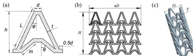
**Figure 1.** Vascular stent model with NPR structure, (a) Arrowhead NPR structure unit; (b) Stent flat developing drawing; (c) Three-dimensional model of stent.
