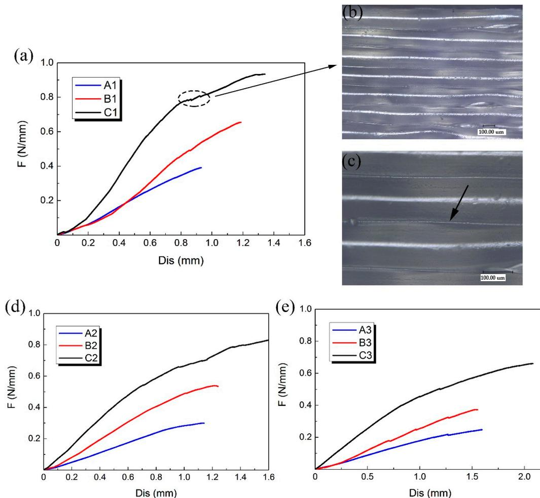
**Figure 8.** Radial force (per unit length) versus radial displacement curves for different wall thickness of 3D-printed PLA vascular stents and the digital microscope images of stent surface, (a) PLA vascular stents with 12 mm stent diameter; (b) Digital microscope image of PLA stent surface magnified 200 times; (c) Digital microscope image of PLA stent surface magnified 500 times; (d) PLA vascular stents with 15 mm stent diameter; (e) PLA vascular stents with 18 mm stent diameter.
