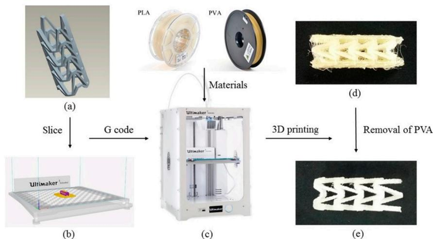
**Figure 2.** 3D printing process of PLA vascular stent, (a) The three-dimensional model of vascular stent; (b) The Cura software interface; (c) The PLA, PVA filaments and Ultimaker 3 Extended 3D printer; (d) The PLA vascular stent with PVA support material; (e) The PLA vascular stent removed PVA material.
