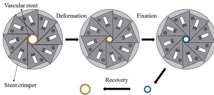
Figure 5. SME experimental process of PLA vascular stent.
