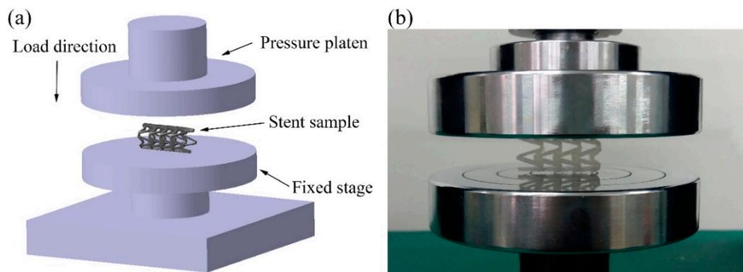
**Figure 4.** Compression experiment of PLA vascular stents, (a) the diagram of loading test setup; (b) stent sample in the test.
