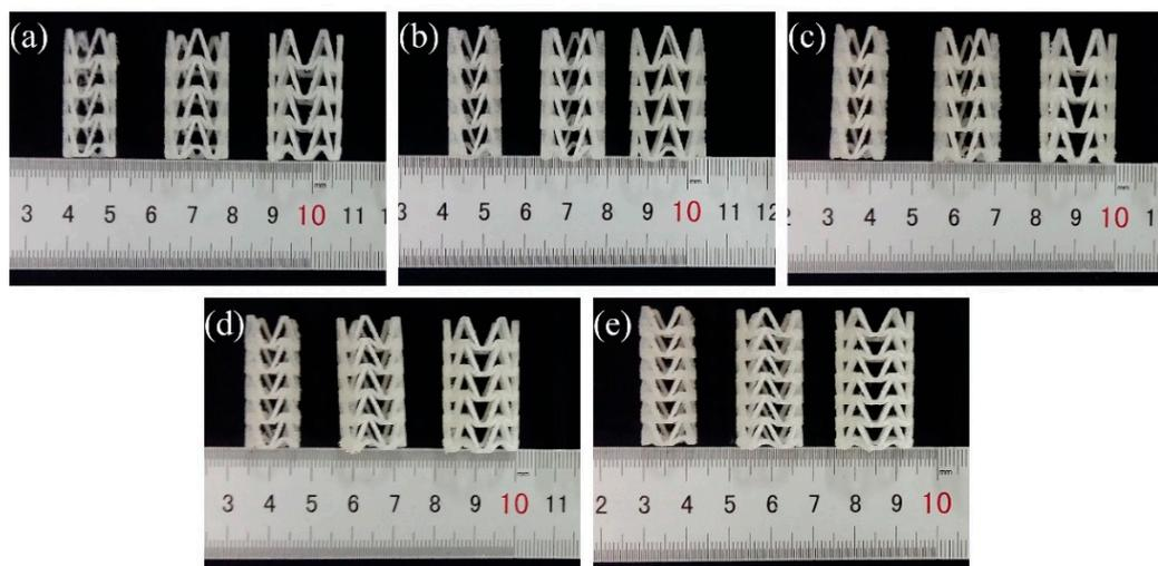
**Figure 3.** 3D-printed PLA vascular stents, from (a–e) are 3D-printed PLA vascular stents of A, B, C, D and E group respectively.
