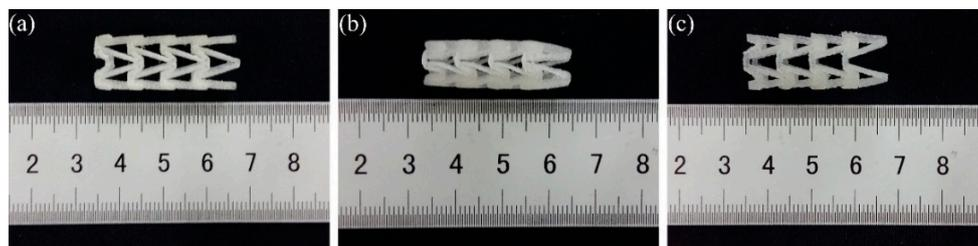
Figure 6. Shape change of numbered B1 3D-printed PLA vascular stent with NPR structure, (a) Original PLA stent; (b) Crimped PLA stent; (c) Recovery PLA stent.
