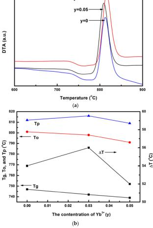
**Figure 1.** (a) Differential Thermal Analysis (DTA) curves of  $Tm^{3+}/Yb^{3+}$  co-doped La<sub>2</sub>O<sub>3</sub>-Nb<sub>2</sub>O<sub>5</sub>-Ta<sub>2</sub>O<sub>5</sub> (LNT) glasses with different contents of Yb<sup>3+</sup> ions; (b) The relationship between the values of T<sub>g</sub>, T<sub>o</sub>, T<sub>p</sub>,  $\Delta$ T, and Yb<sup>3+</sup> content.
