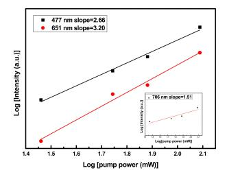
**Figure 3.** The log-log plot of the emission intensity centered around 477, 651, and 706 nm versus the pump power of  $\text{Tm}^{3+}/\text{Yb}^{3+}$  co-doped LNT glasses with y = 0.03.
