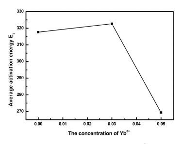
**Figure 5.** The relationship between the average activation energy and  $Yb^{3+}$  concentration in  $Tm^{3+}/Yb^{3+}$  co-doped LNT glasses.
