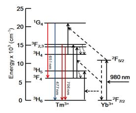
**Figure 4.** Schematic diagram of upconversion luminescence mechanism in Tm<sup>3+</sup>/Yb<sup>3+</sup> co-doped LNT glasses excited at 976 nm laser.
