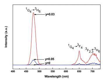
**Figure 2.** Upconversion luminescence spectra of  $Tm^{3+}/Yb^{3+}$  co-doped LNT glasses with different  $Yb^{3+}$  contents pumped at 976 nm laser.
