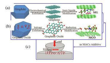
**Figure 5.** The preparation and tribological properties tests of modified graphene (MG) and modified graphene oxide (MGO). (**a**,**b**) Modified graphene (MG) and modified graphene oxide (MGO) were prepared using alkyl imidazolium ionic liquids by electrochemical exfoliation and solvent exfoliation, respectively. (**c**) Schematic of tribological properties tests of MGO and MG. Reproduced with permission from reference Fan et al. [92], Copyright 2015, Elsevior.
