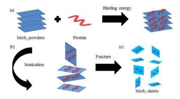
**Figure 8.** Schematic of protein-induced super-thin MoS<sub>2</sub> flakes. (**a**) Step 1: Protein are strongly adsorbed on MoS<sub>2</sub> surfaces via binding energy. (**b**) Step 2: MoS<sub>2</sub> flakes are exfoliated via ultra-sonication. (**c**) Step 3: Layer-by-layer fracture of MoS<sub>2</sub> flakes takes place gradually. Reproduced with permission from reference Liu et al. [121], Copyright 2016, RSC Advances.
