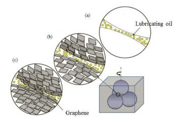
**Figure 4.** Schematic of the four-ball friction test. (a) Friction diagram of pure lubricating oil. (b) Represents optimal concentration of graphene in oil. (c) Represents excessive concentration of graphene in oil. Reproduced with permission from reference Zhang et al. [83], Copyright 2011, IOP.
