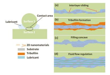
**Figure 1.** Anti-friction and anti-wear mechanisms of 2D materials. (**a**) entering the contact area of sliding surfaces, (**b**) tribofilm forming, (**c**) filling the pits and gaps of contact area, (**d**) affecting the fluid drag and viscosity. Reproduced with permission from reference Xiao et al. [39], Copyright 2017, Elsevier.
