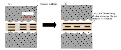
**Figure 7.** Schematic of the water lubrication mechanism of liquid graphene. (**a**) The individually dispersed graphene sheet on the contact surface; (**b**) during the sliding process, the individually dispersed graphene sheets can be rearranged on the surface to form a composite protective film, which effectively reduces friction and wear. Reproduced with permission from reference Yang et al. [115], Copyright 2017, Elsevier.
