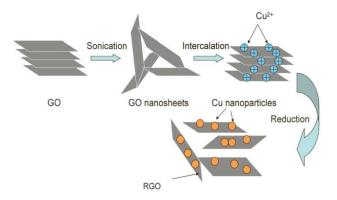
**Figure 6.** Preparation of RGO/Cu nanoparticle composites. Step 1: Graphene oxide (GO) nanosheets are exfoliated to lots of single GO nanosheets and the metal cations are inserted on single GO nanosheets. Step 2: Cu nanoparticles are generated on the action of strong reductant. Reproduced with permission from reference Zhang et al. [98], Copyright 2013, RSC Advances.
