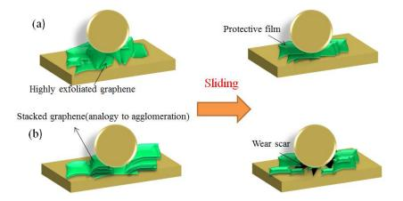
**Figure 3.** The lubrication mechanisms of graphene in different degrees of peeling. (a) During the sliding process, graphene with higher exfoliation restacks to lamellar a protective film. (b) The stacked graphene layers are prone to being damaged, and further appear as a wear scar. Reproduced with permission from reference Zhao et al. [73], Copyright 2018, Elsevior.
