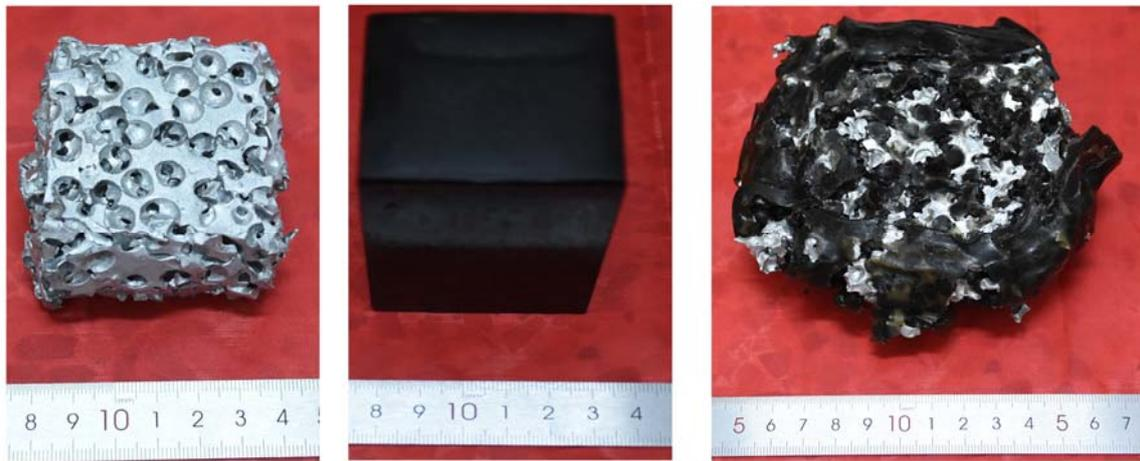
Figure 3. Deformed SCPA, PU and SCPA-PU composites specimens after uniaxial compression tests.
