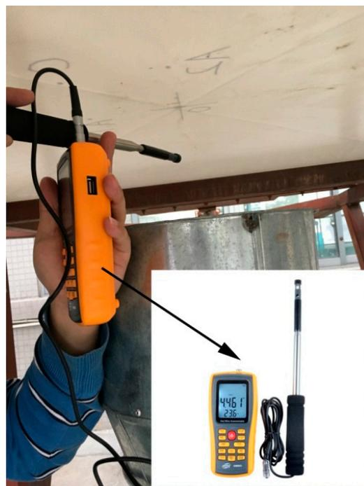
**Figure 6.** Digital velocity measurement.
