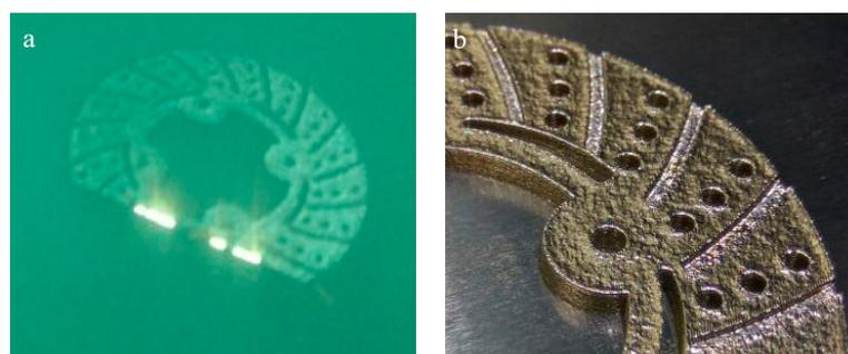
**Figure 3.** (a) Development of brake disc in EOS M-290 and (b) Disc brake developed by DMLS.
