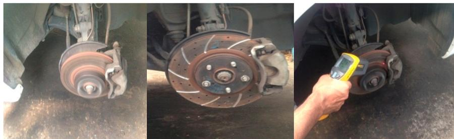
**Figure 7.** Temperature recording on modified brake disc surface with FLUKE IR thermometer.
