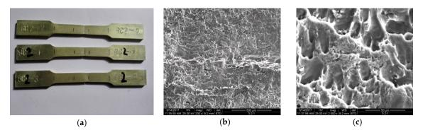
**Figure 7.** Fracture of the specimens: (**a**) mechanical testing of the weld joints; (**b**) fracture surface of tension specimen; (**c**) fracture surface of tension specimen.
