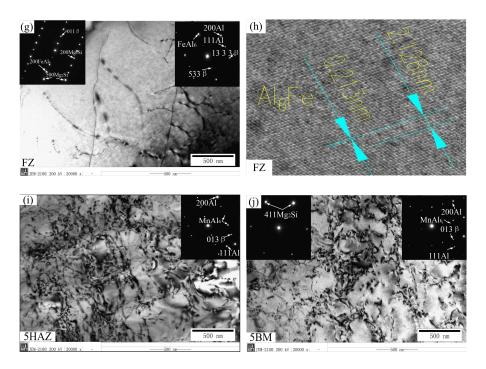
**Figure 9.** TEM study of the microstructure of different parts of the two alloys in the weldment: (**a–c**) microstructure of the base metal (7BM); (**d–f**) microstructure of the heat-affected zone (7HAZ) adjacent to the base metal; (**g**,**h**) microstructure of the fusion zone; (**i**) microstructure of the heat-affected zone (5HAZ) adjacent to the base metal; (**j**) microstructure of the base metal (5BM).
