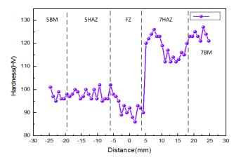
Figure 5. Micro-hardness across the weld.
