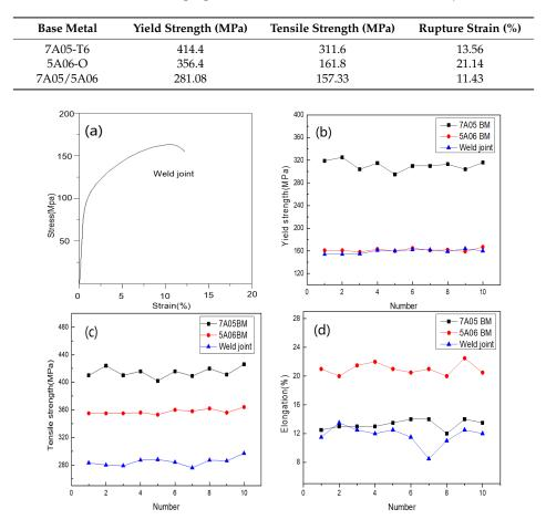
Table 2. Mechanical properties of the 7A05BM, 5A06BM and weld joint.
