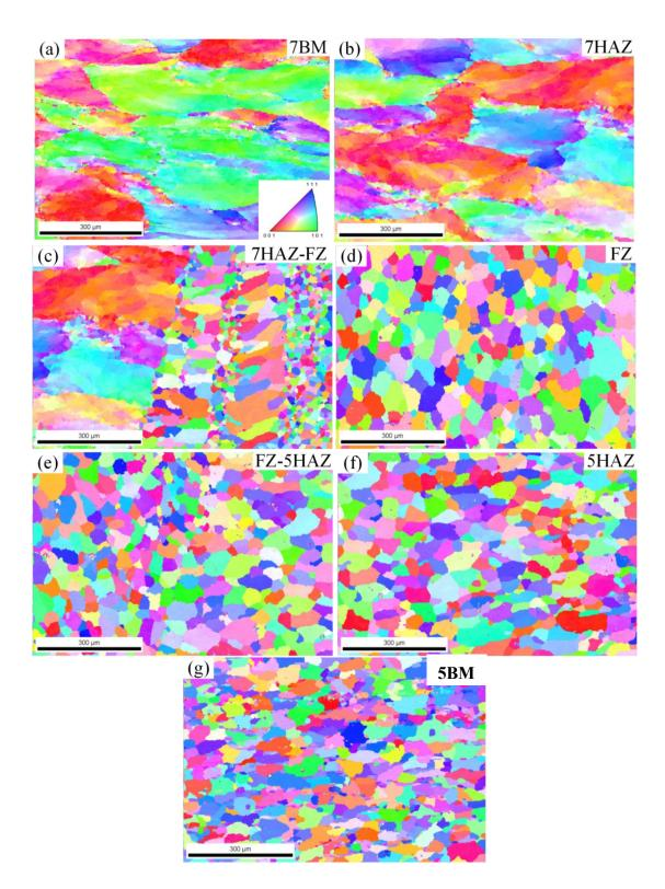
**Figure 8.** EBSD study of the microstructures of different parts of the two alloys in the weldment. The parts correspond to the EBSD images are indicated in the top right corners. (a) 7BM; (b) 7HAZ; (c) 7HAZ-FZ; (d) FZ; (e) FZ-5HAZ; (f) 5HAZ; (g) 5BM.
