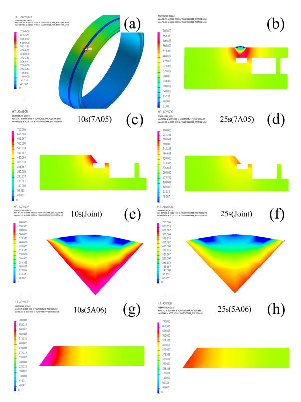
**Figure 11.** Temperature field distributions: (**a**) simulation of temperature field distribution of welded joints; (**b**) temperature distribution of welded joint profiles; (**c**–**d**) 7A05BM profile temperature field distribution; (**d**,**e**) weld profile temperature field distribution; (**g**,**h**) 5A06BM profile temperature field distribution.
