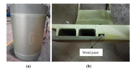
**Figure 3.** Physic structures of welded sample: (**a**) the 5A06-O/7A05-T6 welded sample; (**b**) the cross section of 5A06-O/7A05-T6 welded joint.
