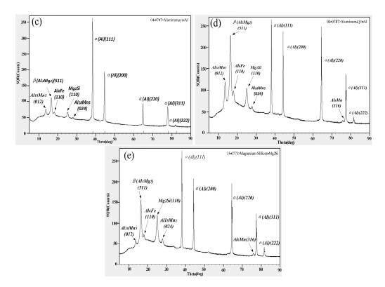
**Figure 10.** XRD study of the microstructure of different parts of the two alloys in the weld joint: (a) microstructure of the base metal (7BM); (b) microstructure of the heat-affected zone adjacent to the base metal (7HAZ); (c) microstructure of the fusion zone; (d) microstructure of the heat-affected zone adjacent to the base metal (5HAZ); (e) microstructure of the base metal (5BM).
