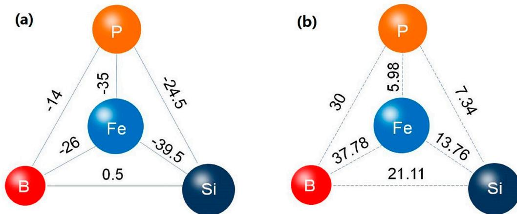
**Figure 5.** Schematic illustration for the mixing enthalpy (a) and mismatch in atomic radius (b) for the Fe-Si-B-P alloy system.
