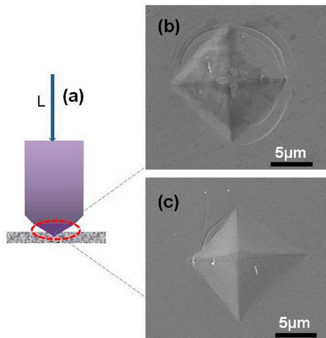
**Figure 12.** Schematic diagram of the Vickers indentation testing (a) and SEM images of indentation marks of the  $\text{Fe}_{80}\text{Si}_9\text{B}_8\text{P}_3$  amorphous ribbon; (b) as-quenched specimen; and, (c) annealed at  $400\text{ }^\circ\text{C}$  for 10 min.
