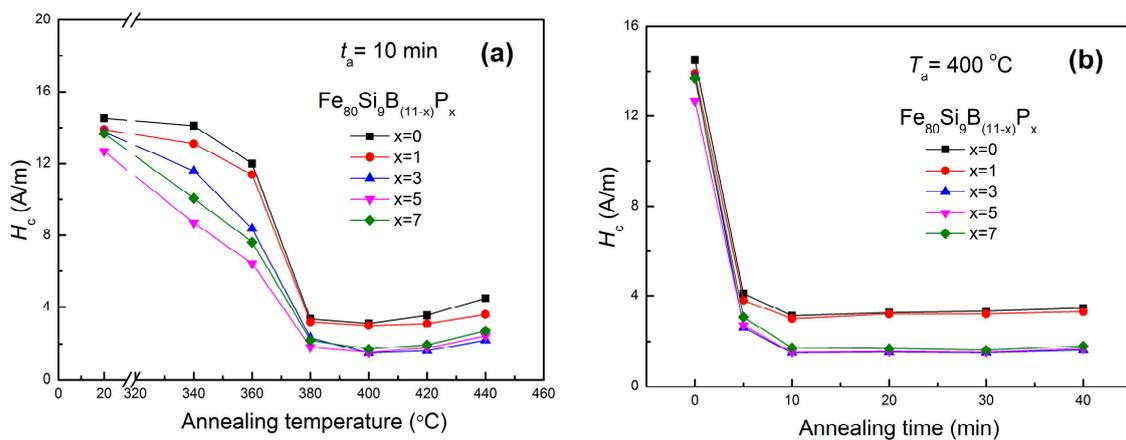
**Figure 7.** Annealing temperature ( $T_a$ ) dependence (a) and annealing time ( $t$ ) dependence (b) of  $H_c$  for  $\text{Fe}_{80}\text{Si}_9\text{B}_{(11-x)}\text{P}_x$  ( $x = 0, 1, 3, 5, 7$ ) amorphous alloys.
