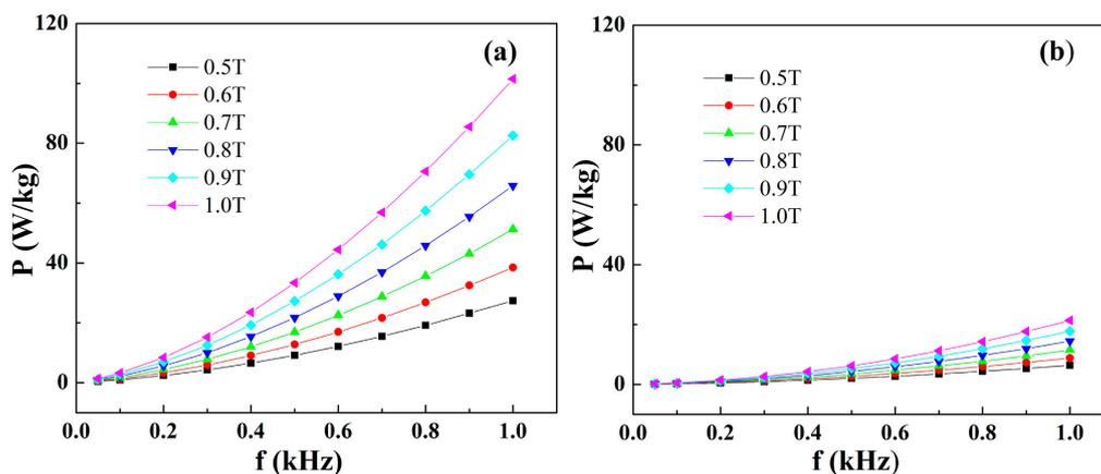
**Figure 9.** Core losses as a function of frequency in different induction; (a) conventional silicon steel (b)  $Fe_{80}Si_9B_8P_3$  amorphous alloys.
