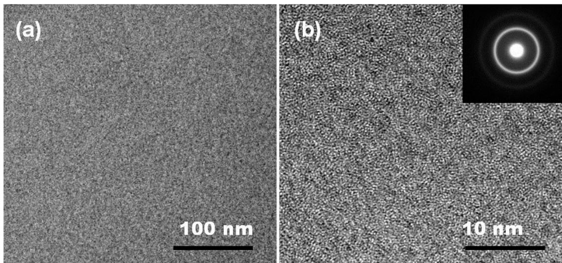
**Figure 4.** The Bright-field TEM images (a) high-resolution TEM (HRTEM) images and (b) corresponding selective area diffraction patterns (inset) of  $\text{Fe}_{80}\text{Si}_9\text{B}_8\text{P}_3$  sample with a ribbon thickness of 65  $\mu\text{m}$ .
