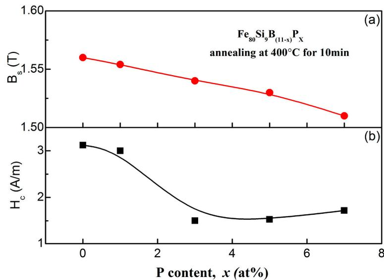
**Figure 8.** Changes of  $H_c$  (a) and  $B_s$  (b) for  $Fe_{80}Si_9B_{(11-x)}P_x$  ( $x = 0, 1, 3, 5, 7$ ) amorphous ribbons as a function of P content annealed at 400 °C for 10 min.
