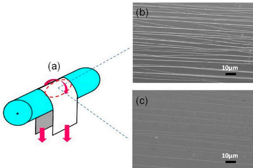
**Figure 11.** Schematic diagram of the bending test (a) and SEM images obtained from the top surface of the bent  $\text{Fe}_{80}\text{Si}_9\text{B}_8\text{P}_3$  alloy ribbons; (b) as-quenched specimen; and, (c) annealed at  $400\text{ }^\circ\text{C}$  for 10 min.
