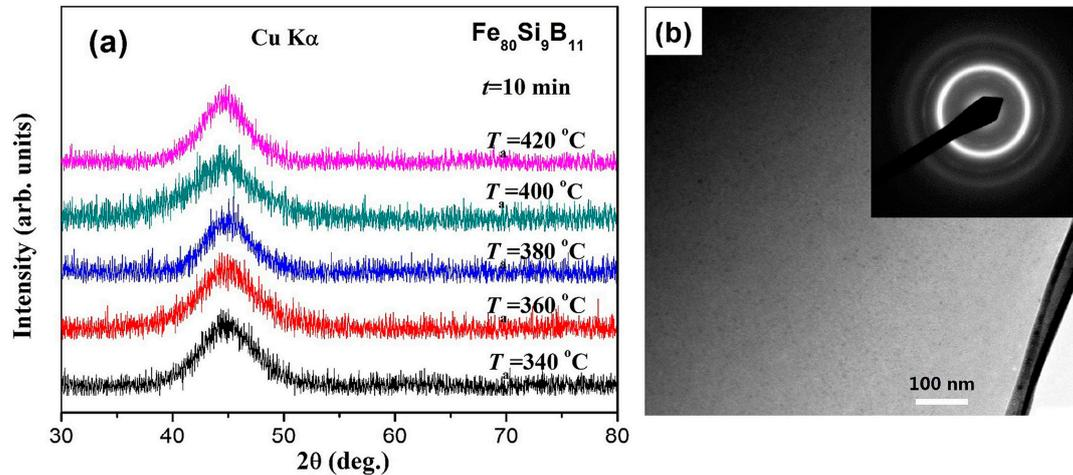
**Figure 10.** (a) X-ray diffraction (XRD) patterns of the as-spun  $\text{Fe}_{80}\text{Si}_9\text{B}_{11}$  samples annealed at different temperatures for 10 min; (b) The Bright-field TEM images and corresponding selective area diffraction patterns (inset) of  $\text{Fe}_{80}\text{Si}_9\text{B}_{11}$  sample annealed at 420 °C for 10 min.
