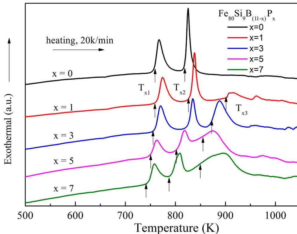
**Figure 6.** DSC curves of the as-spun  $\text{Fe}_{80}\text{Si}_9\text{B}_{(11-x)}\text{P}_x$  ( $x = 0, 1, 3, 5, 7$ ) amorphous ribbons at a heating rate of 20 K/min.
