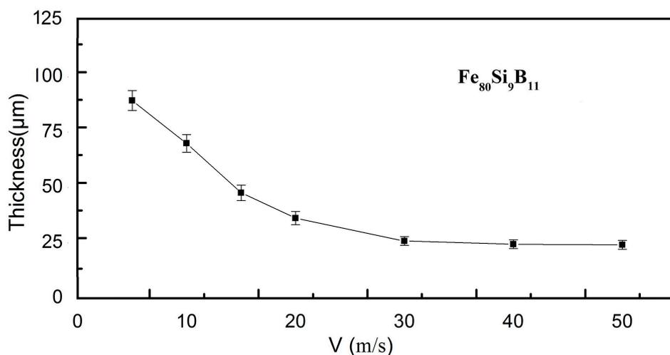
**Figure 2.** Variation of the thickness for  $\text{Fe}_{80}\text{Si}_9\text{B}_{11}$  as-spun ribbons as a function of the tangential wheel speed.
