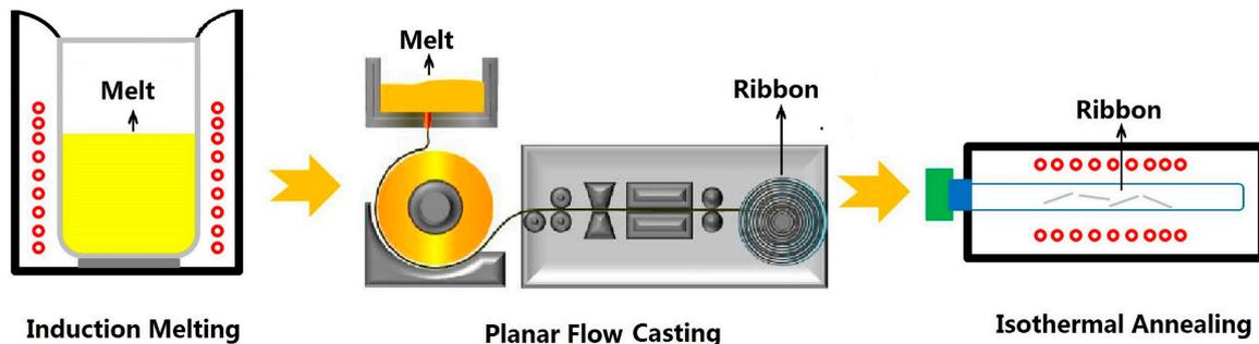
**Figure 1.** The schematic formation process for the  $\text{Fe}_{80}\text{Si}_9\text{B}_{(11-x)}\text{P}_x$  ( $x = 0, 1, 3, 5, 7$ ) amorphous soft magnetic alloys.
