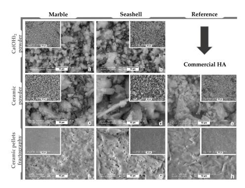
**Figure 1.** Representative micrographs for marble, seashell and reference material derived products: Ca(OH)<sub>2</sub> (**a**,**b**), Ceramic powder (**c**–**e**), Ceramic pellets fractographic surface (**f**–**h**).
