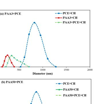
Figure 15. Size distribution of PAA and PCE in CH solution (a: PAA3–PCE; b: PAA50–PCE).
