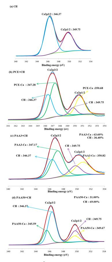
**Figure 12.** Binding energy of Ca<sup>2+</sup> (**a**: CH; **b**: PCE-Ca; **c**: PAA3-Ca; **d**: PAA50-Ca).
