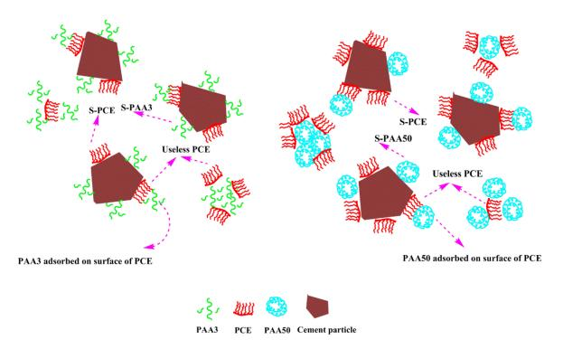
Figure 17. Mechanism model of cement suspension with PCE.
