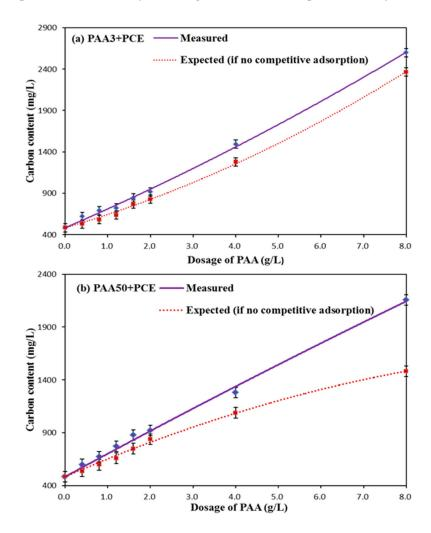
Figure 9. Competitive adsorption between PAA and PCE (1.2 g/L) (a: PAA3–PCE; b: PAA50–PCE).
