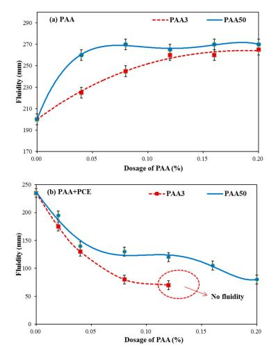
Figure 5. Effect of polymers on fluidity performance of cement paste (a: PAA; b: PAA-PCE).
