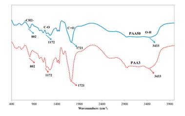
Figure 3. FTIR spectra of PAA.
