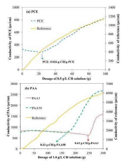
Figure 11. Conductivity of polymers with addition of CH solution (a: PCE; b: PAA).
