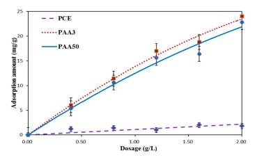
Figure 8. Adsorption amount of PAA and PCE.
