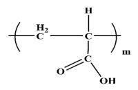
Figure 2. Molecular structure of PAA.
