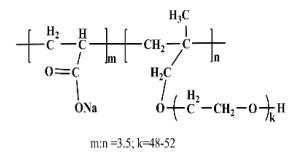
Figure 1. Molecular structure of PCE.
