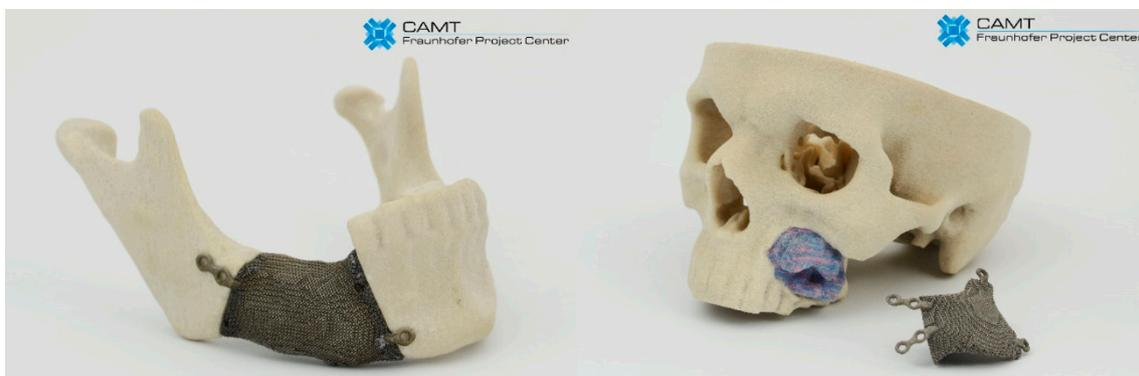
**Figure 14.** Examples of custom-made implants made of Ti6Al7Nb alloy filled with BFS.
