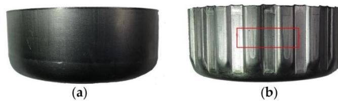
**Figure 9.** Surface appearance before and after the clutch forming process without vibration: (a) Before forming; (b) After forming.
