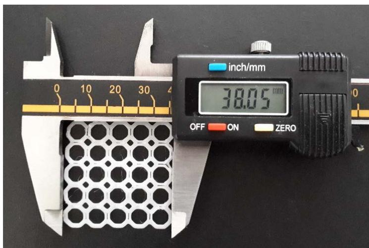
**Figure 1.** Digital image of the 3D printed PCL scaffold measured with a digital caliper.
