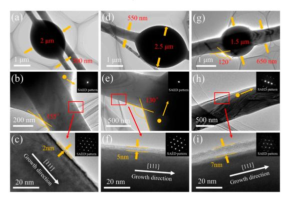
**Figure 7.** Typical transmission electron microscopy (TEM) images, high-resolution transmission electron microscopy (HRTEM) lattice images, and SAED patterns of the as-prepared samples: (**a**–**c**) 1200 °C; (**d**–**f**) 1300 °C; (**g**–**i**) 1400 °C.
