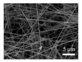
**Figure 6.** SEM images of the as-achieved products (firing at 1200  $^{\circ}$ C) after hydrofluoric acid (HF) treatment.
