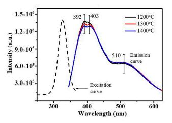
Figure 8. Emission spectra of SiC/SiO<sub>2</sub> heterojunctions synthesized at different temperatures.
