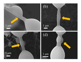
**Figure 10.** SEM images of the liquid SiO<sub>2</sub> movement of the as-prepared samples after firing at 1400 °C. (a) SiO<sub>2</sub> bean; (b) Migration of SiO<sub>2</sub> droplet; (c) shrinkage of SiO<sub>2</sub> droplet; (d) SiO<sub>2</sub> bean
