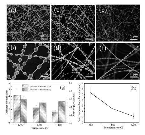
**Figure 2.** Scanning electron microcopy (SEM) images of the as-achieved products as a function of the firing temperature, (**a**,**b**) 1200 °C; (**c**,**d**) 1300 °C; (**e**,**f**) 1400 °C; (**g**) histogram for the diameter of the beans and chains in a necklace-like structure; (**h**) line chart representing the ratio of the beans' diameter to the chains' diameter.
