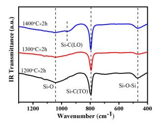
Figure 4. Fourier-transform-infrared spectroscopy (FT-IR) absorbance spectrum of the as-received samples.
