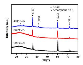
Figure 3. X-ray diffraction (XRD) patterns of the as-received samples.
