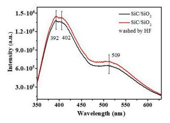
Figure 9. Emission spectra of SiC/SiO<sub>2</sub> heterojunctions after HF treatment.
