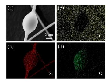
**Figure 5.** Mapping the energy dispersive X-ray spectroscopy (EDS) patterns of the  $SiC/SiO_2$  heterojunctions synthesized at 1200 °C: (a) SEM images of the products; (b) C element; (c) Si element; (d) O element.
