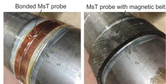
**Figure 4.** Photograph of pipe and MsT probe used for harmonic generation experiments.
