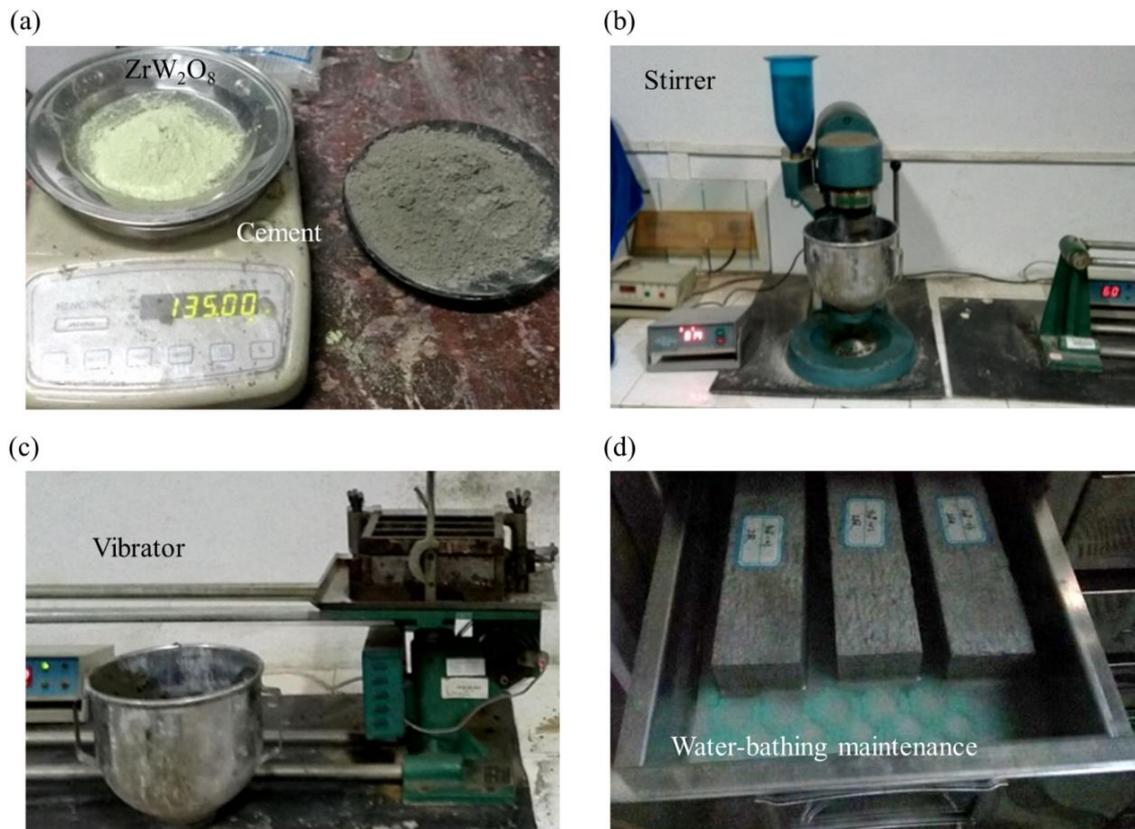
**Figure 1.** Fabrication of cementitious composites including synthesis, molding, hydration, solidification, and maintenance. (a)  $\text{ZrW}_2\text{O}_8$  and cement are the main ingredients of cementitious composites; (b) The stirrer is used to blend uniformly all the ingredients; (c) The vibrator is employed to exclude pores inside and densify composites; (d) Specimens are placed, hydrate and solidify in a water-bathing maintenance environment.
