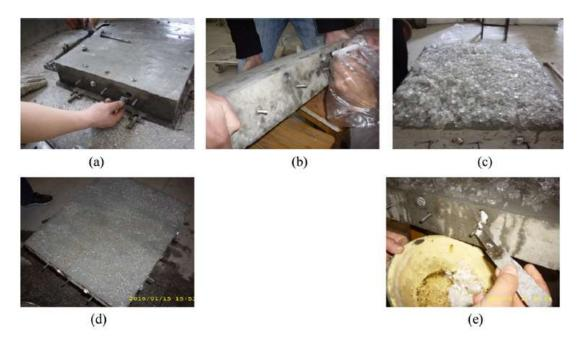
**Figure 17.** The simulation test is carried out under low temperature. (a) Injecting entrance design of PCM; (b) injecting PCM; (c) simulation of surface ice-snow condition; (d) melting ice conditions of surface; (e) phase change completion of PCM [31].
