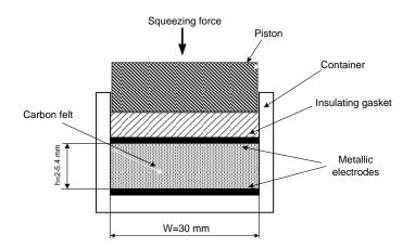
Figure 7. The cell for electrical conductivity measurements.
