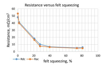
Figure 8. Resistance of a dry felt versus volume compression.
