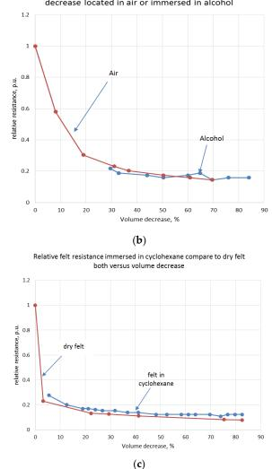
Relative felt resistance diminishing versus volume decrease located in air or immersed in alcohol
