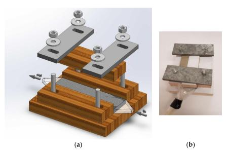
Figure 2. (a) 3D drawing and (b) a view of experimental cell for hydraulic permeability measurements.
