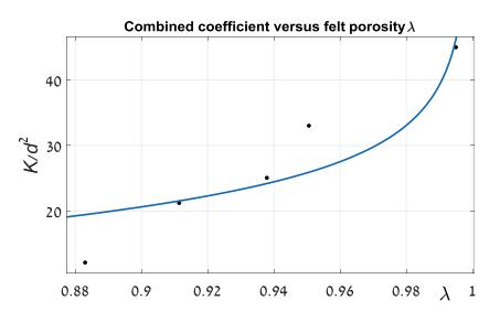
**Figure 5.** Combined coefficient  $k/d^2$  versus felt porosity  $\lambda$ .
