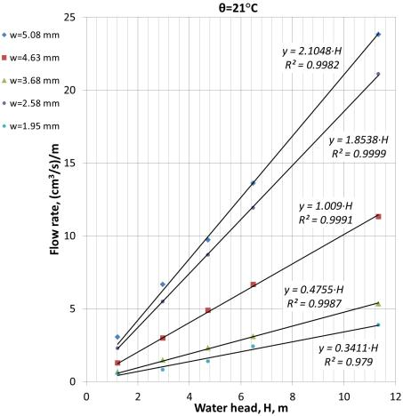
Flow rate versus water head for different felt widths, water
