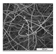
Figure 1. A magnified picture of the CF structure.
