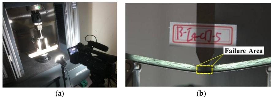
**Figure 3.** Three-point bending testing. (a) Light transmittance method; (b) Failure zone.
