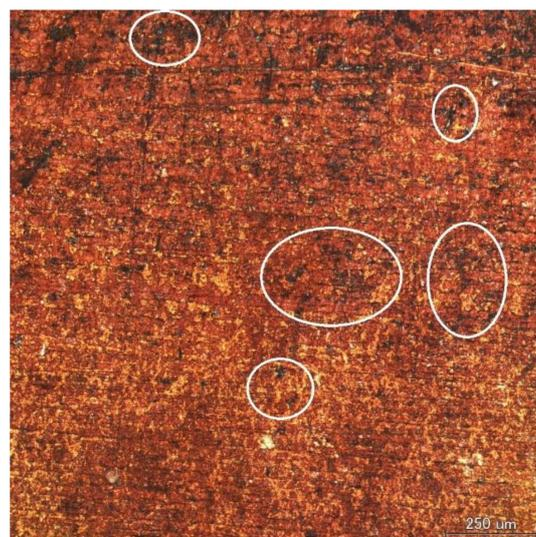
**Figure 2.** Surface observations of Cu tube specimen immersed in  $10^3$  ppm  $\text{Cu}(\text{HCOO})_2$  after 10 days immersion.
