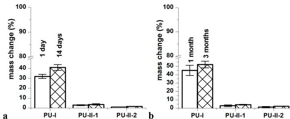
Figure 5. Distilled water (a) and PBS (b) sorption of obtained PURs after selected incubation time-points.
