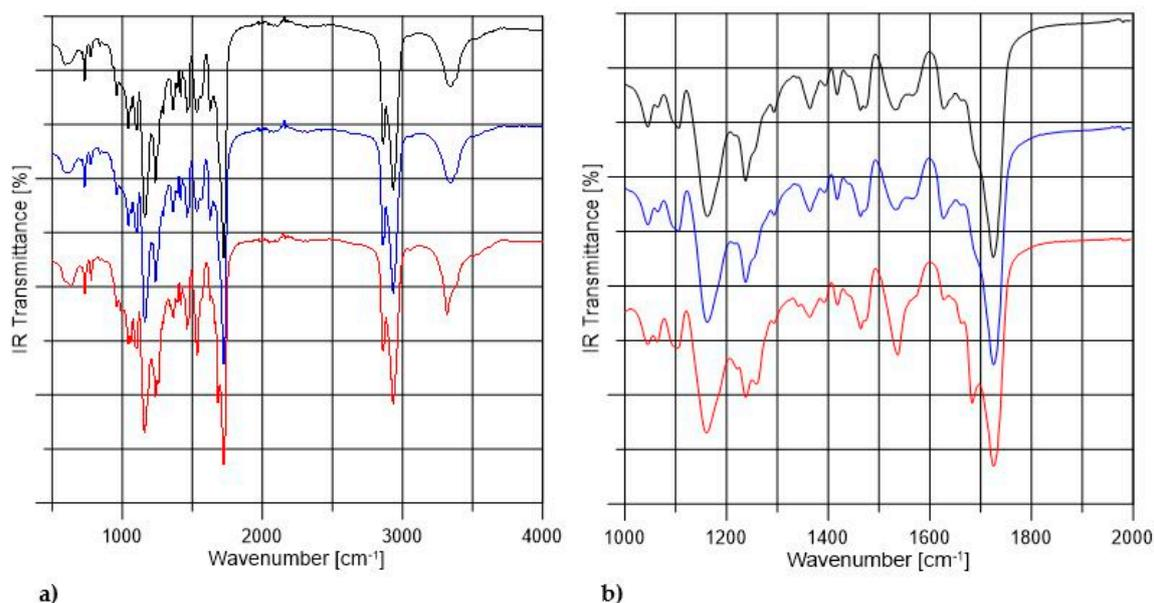
**Figure 2.** The FTIR spectra of non-crosslinked (black) and PVA-crosslinked PURs (blue and red respectively for 1 wt % and 2 wt % of PVA) in the range between 500–4000  $\text{cm}^{-1}$  (a) and in the range of 1000–2000  $\text{cm}^{-1}$  (b).
