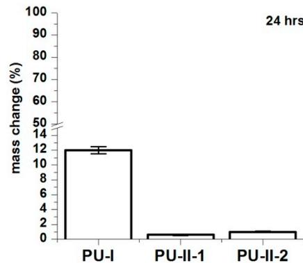
Figure 4. Canola oil sorption noted for PU-I, PU-II-1, PU-II-2 after 24 h of incubation.
