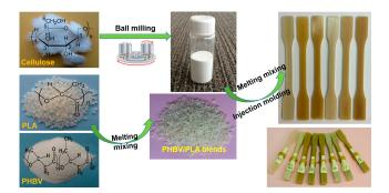
**Figure 1.** Schematic of fabricating the ternary cellulose-modified poly(hydroxybutyrate-co-hydroxyvalerate) (PHBV)/polylactide (PLA) composites.
