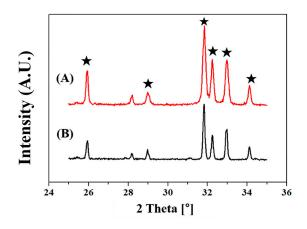
**Figure 3.** Representative XRD patterns of (**A**) as-received HA powders and (**B**) HA microspheres synthesized using spray drying ( $\bigstar$ : HA phase).
