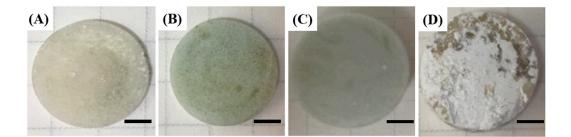
**Figure 4.** Representative optical images of poly(methyl methacrylate) (PMMA)/HA composites produced using the HA microspheres with various HA contents of (**A**) 5 vol %; (**B**) 20 vol %; (**C**) 40 vol %; and (**D**) composite produced using the HA powders with an HA content of 20 vol % (Scale bar = 3 mm).
