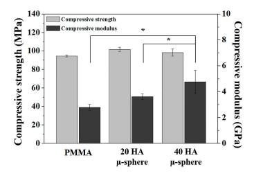
**Figure 6.** Compressive strengths and compressive modulus of PMMA/HA composites with various HA contents of 20 vol % (20 HA  $\mu$ -sphere) and 40 vol % (40 HA  $\mu$ -sphere) and PMMA bone cement containing barium sulfate (PMMA) (\* p < 0.05).
