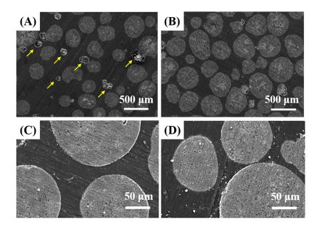
**Figure 5.** Representative SEM images of PMMA/HA composites produced using the HA microspheres with various HA contents of 20 vol % (**A**,**C**) and 40 vol % (**B**,**D**), showing distribution of the HA microspheres in the PMMA matrix (**A**,**B**) and interfacial bonding between the HA microspheres and PMMA (**C**,**D**). Yellow arrows indicate voids formed during the grinding process for SEM observations.
