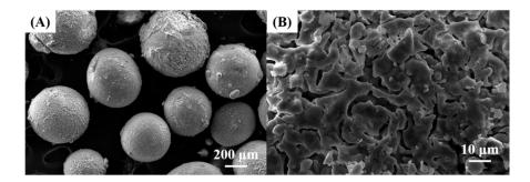
**Figure 2.** Representative SEM images of synthesized hydroxyapatite (HA) microspheres displaying (**A**) well-defined spherical shape and (**B**) relatively rough surface.
