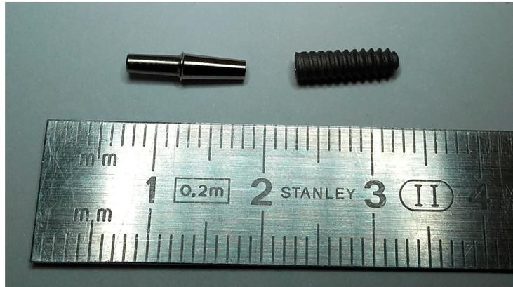
**Figure 10.** Image of the implant-abutment assembly prototype made of  $\text{Ti}_{40}\text{Zr}_{10}\text{Cu}_{36}\text{Pd}_{14}$  BMG, machined in the same conditions as Ti-6Al-4V Extra Low Interstitial (ELI) assemblies.
