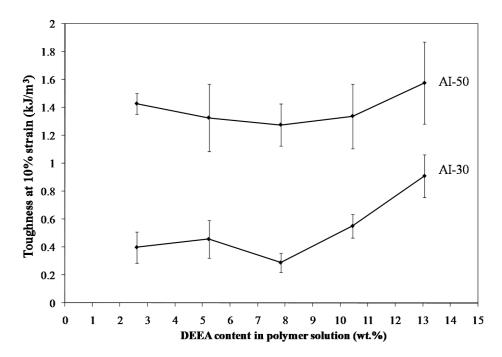
**Figure 5.** Toughness at 10% strain of 5 wt. % Na<sup>+</sup>-MMT/2.5 wt. % AI-30 composites as a function of amine concentration.
