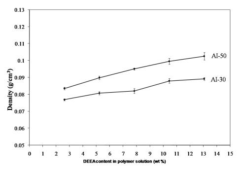
**Figure 3.** Change in density of 5 wt. % Na<sup>+</sup>-MMT/2.5 wt. % AI-30 composites as a function of amine concentration.
