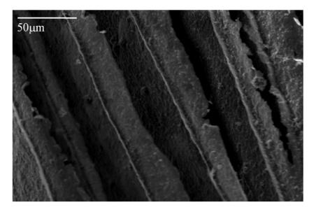
**Figure 2.** SEM (Scanning Electron Microscope) image of the microstructure of a 5 wt. % Na<sup>+</sup>-MMT/2.5 wt. % (Nanocor Inc. PGW grade, Chicago, IL, USA) AI-30 composite with 2 equivalents of amine.
