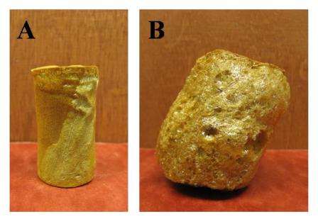
Figure 6. Image of 5 wt. % Torlon<sup>®</sup> AI-50 materials with (A) 6 and (B) 10 equivalents of amine.
