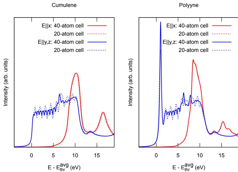
**Figure S4.** NEXAFS spectrum of cumulenes (left) and polyynes (right) computed with a 20-atom and 40-atom simulation supercell. One atom per cell is excited. Polarization directions are taken with  $x$  along the chain axis and  $y, z$  orthogonal to it.
