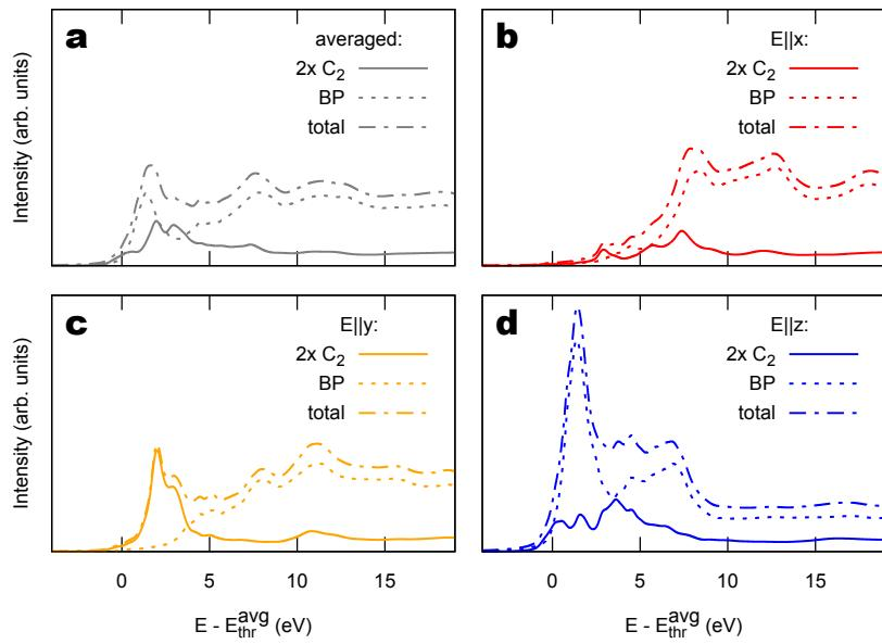
**Figure S3.** Decomposition of the NEXAFS spectrum of bBEBP/Au(111) embedding a Au adatom on contributions by the  $\text{sp}^2$  biphenyl part (BP) and the  $\text{sp}^1$  chains ( $\text{C}_2$ ). (a) Spectrum averaged over the polarizations. (b) In-plane electric field along the polymer axis  $x$  and (c) orthogonal to it,  $y$ ; (d) out-of-plane electric field,  $z$ . See Figure S2a for the definition of  $x, y, z$  axes.
