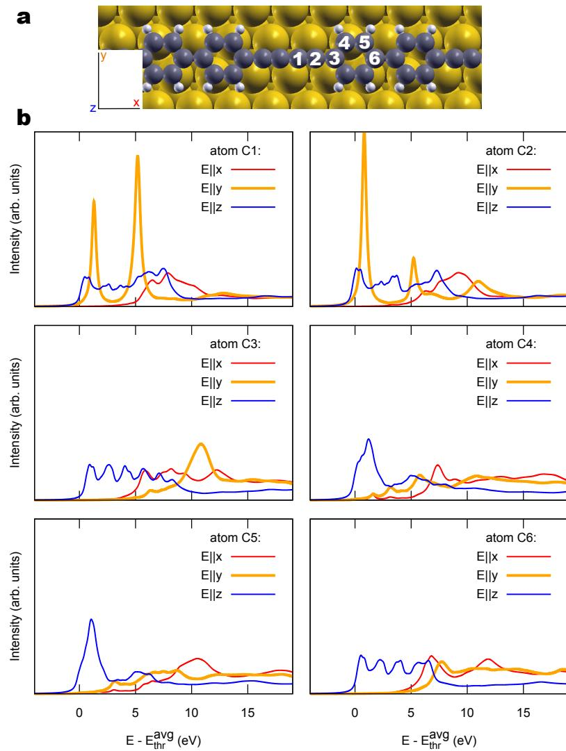
**Figure S1.** (a) Structural model and inequivalent carbon atoms in bBEBP/Au(111). (b) Decomposition of the NEXAFS spectrum of bBEBP/Au(111) into the individual initial-state contributions, as numbered in panel (a).
