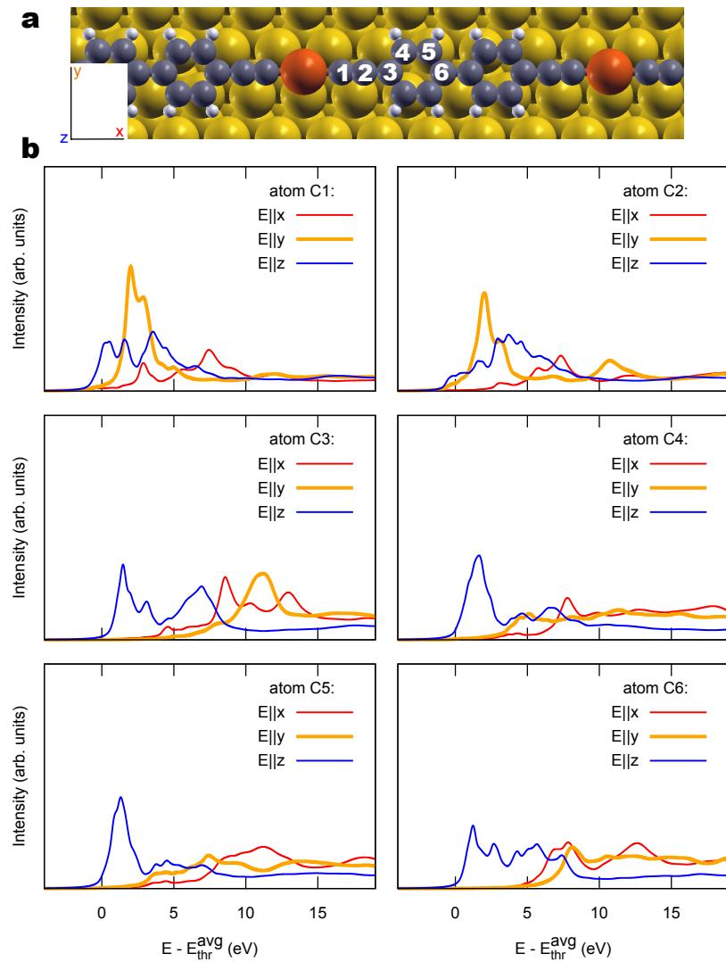
**Figure S2.** (a) Structural model and inequivalent carbon atoms in bBEBP/Au(111) embedding a Au adatom (red) in between two organic units. (b) Decomposition of the corresponding NEXAFS spectrum into the individual initial-state contributions, as numbered in panel (a).
