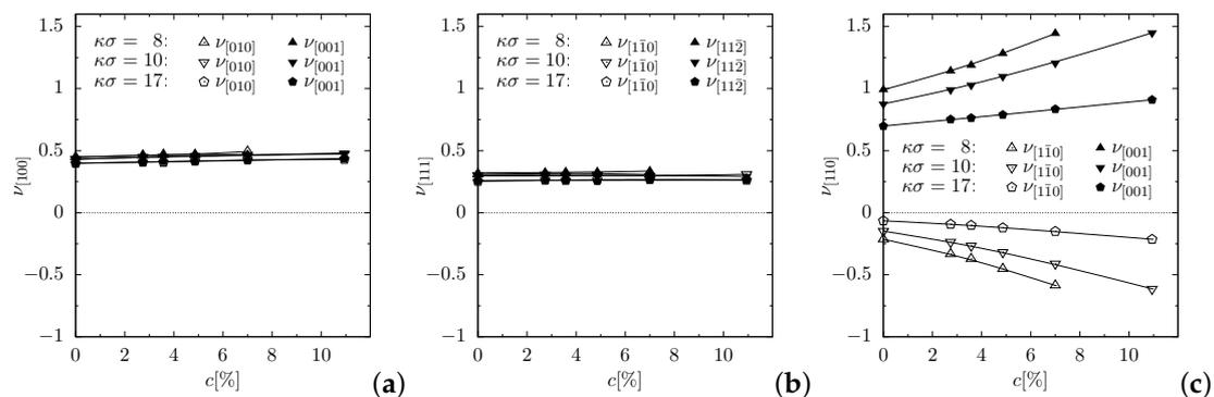
**Figure 5.** Poisson’s ratio of Yukawa crystals with nanochannels in the main crystallographic directions with respect to the concentration: (a)  $[100]$ ; (b)  $[111]$ ; and (c)  $[110]$ .
