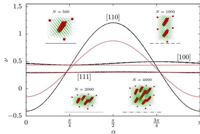
**Figure 4.** Poisson’s ratio in three crystallographic directions for various size of the system ( $N = 500, 1000, 2000,$  and  $4000$ ) as a function of the angle  $\alpha$  (with  $c = 7\%$ ,  $p^* = 100$ ,  $\kappa\sigma = 10$  and  $\beta\epsilon = 20$ ). Red lines represent Poisson’s ratio in the respective crystallographic directions of the system without nano-inclusions.
