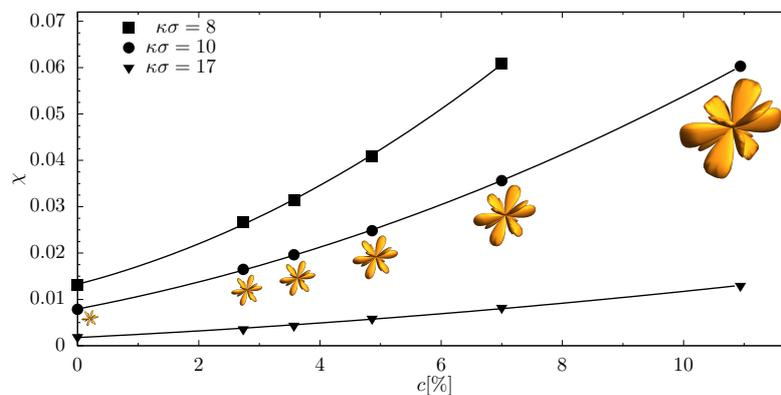
**Figure 7.** Degree of auxeticity with respect to the concentration for various values of screening length. The inserts in the figure show the average absolute value of negative Poisson's ratio (Equation (9)) in all crystallographic directions for  $\kappa\sigma = 10$ . The surface consists of the points that represent  $R(\theta, \phi)$ . All the inserted figures are presented at the same scale.
