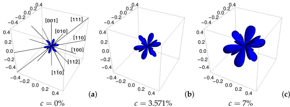
**Figure 6.** Absolute value of the minimal negative Poisson's ratio in all crystallographic directions for Yukawa systems with nanochannels in the  $[111]$ -direction for inverse screening length  $\kappa\sigma = 10$  and various concentrations: (a)  $c = 0\%$ ; (b)  $c = 3.571\%$ ; and (c)  $c = 7\%$ .
