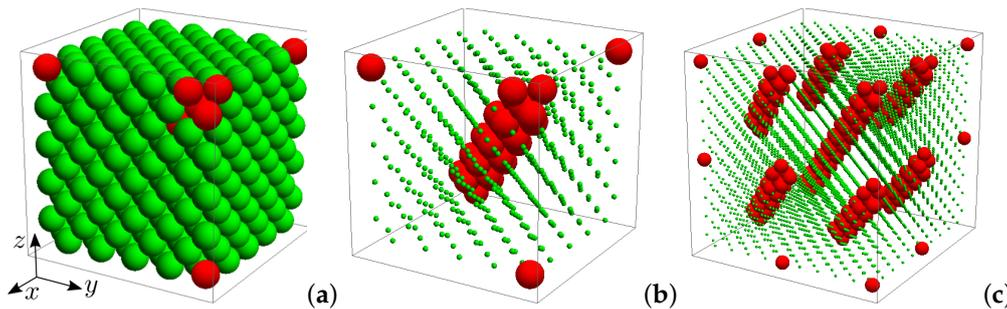
**Figure 1.** The structures of studied crystals with nanochannels in the [111]-crystallographic direction: (a) with green are marked particles which interact via the hard-core repulsive Yukawa pair potential (HCRYP), while red particles represent the hard spheres; (b) to better illustrate the structure of nanochannel, the centers of Yukawa particles are marked by green dots; and (c) periodic boundary conditions result in the structure with periodic array of nanochannels.
