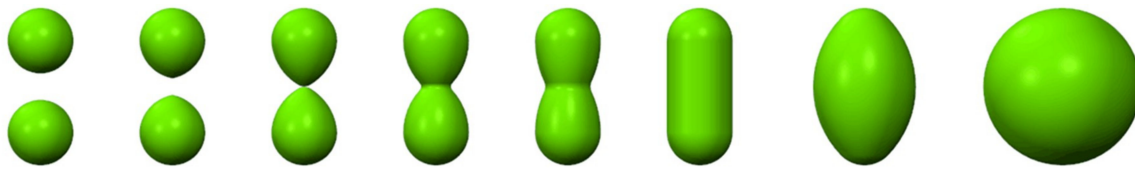
Figure 7. A schematic diagram of the \text{Ag}_3\text{Sn} coarsening following the necking-coalescence during TS cycling.
