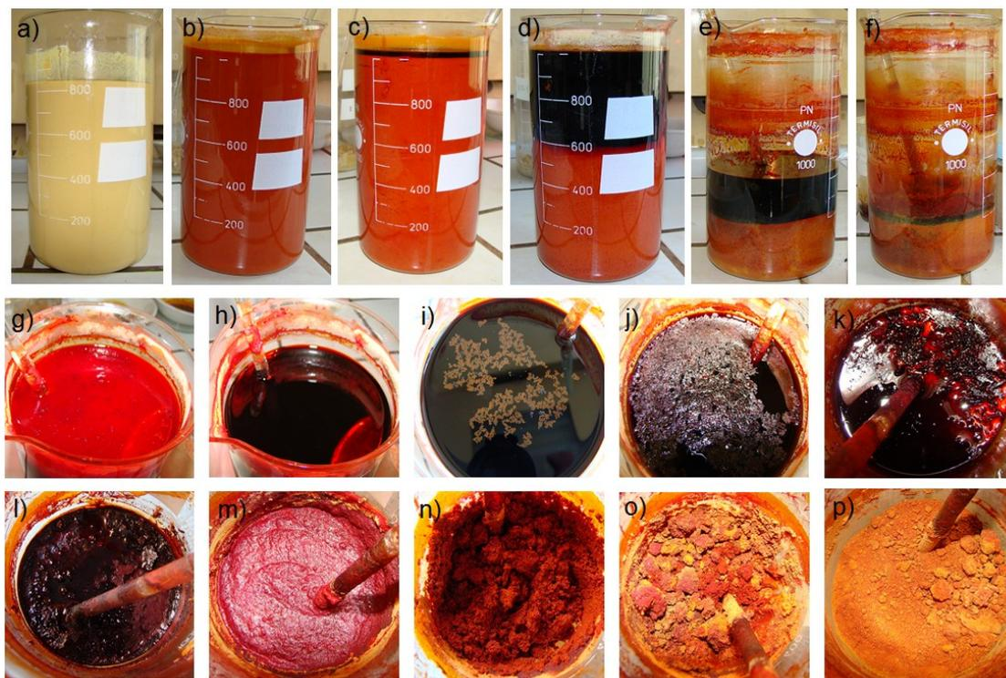
**Figure 1.** The precipitation method of the  $\text{PbFe}_{1/2}\text{Nb}_{1/2}\text{O}_3$  material: (a–f) side view, (g–p) top view. Successive stages of the technological process: (a) mixing ingredients, (b,g) introducing acetylacetone and distilled water, (c–f) and (h–l) the solvent vaporization (as a result of the IR lamp effect on the solution), (m–o) powder formation, (p) powder after completion of drying.
