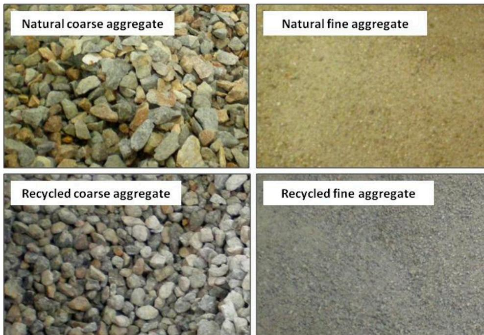
Figure 1. Aggregates used in the experimental work.
