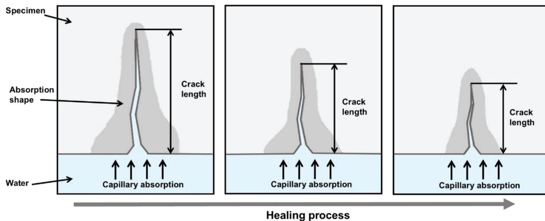
**Figure 3.** Schematic of change in capillary water absorption through crack as healing progresses.
