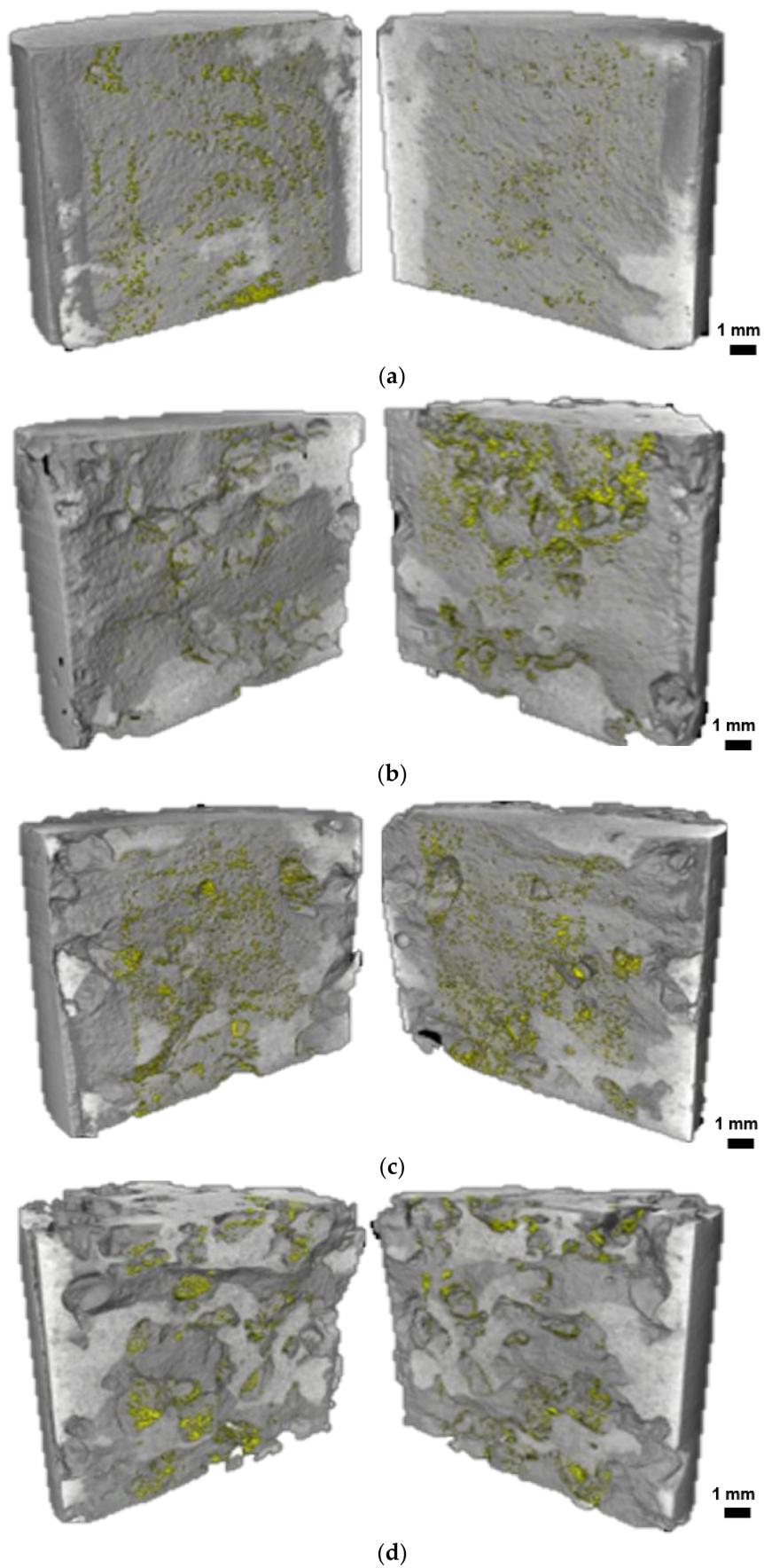
**Figure 13.** Three-dimensional images of split specimens; healing products are shown in yellow (a) REF; (b) S-0.5; (c) S-1.0; and (d) S-1.5 specimens.
