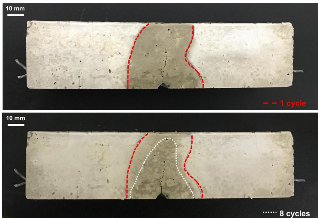
**Figure 7.** Region of water absorption in the S-0.5 specimen at first and eighth cycles during the capillary water absorption test.
