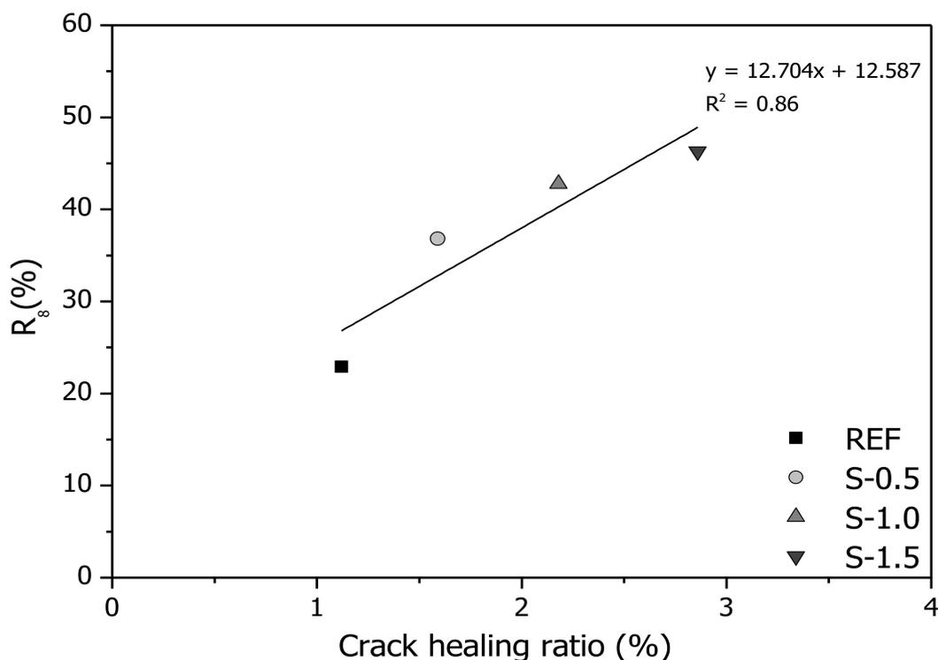
**Figure 15.** Relationship between reduction ratio of initial sorptivity at eighth cycle ( $R_8$ ) and crack healing ratio.
