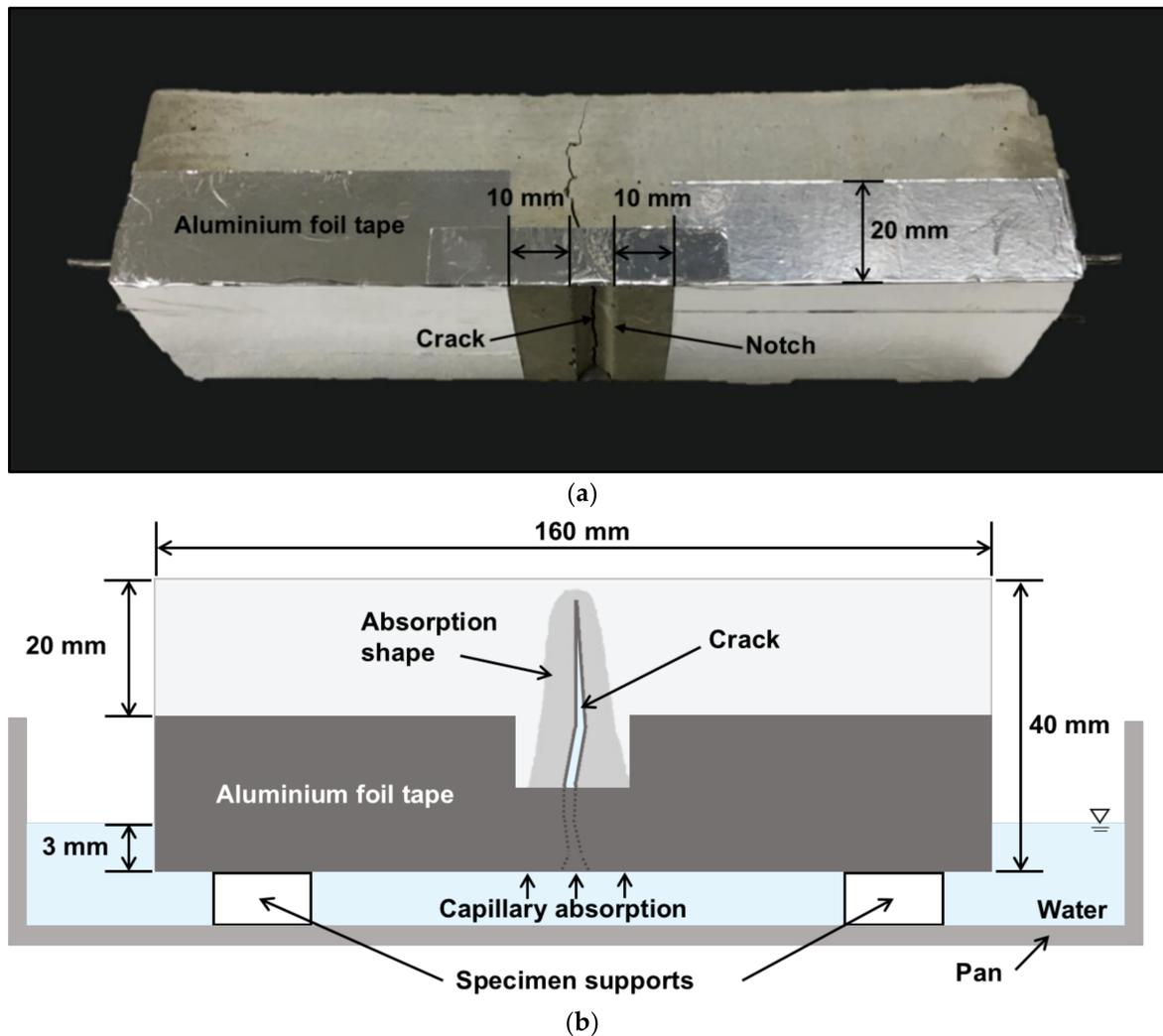
**Figure 4.** (a) Specimen sealed with aluminum foil tape; (b) Illustration of capillary water absorption test.
