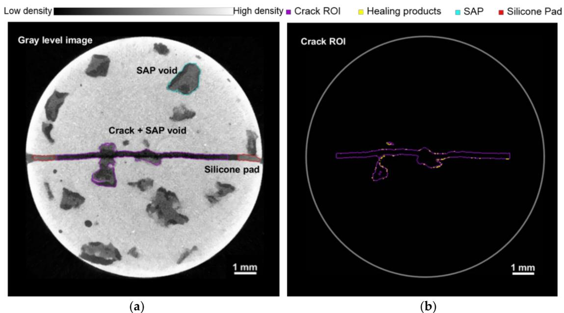
**Figure 10.** (a) Gray-level X-ray micro CT image of specimen. Crack regions of interest (ROI) includes the crack and directly connected SAP voids is shown in purple, the silicone pad in red, and SAP voids in blue; (b) The crack ROI (purple) and healing products (yellow).
