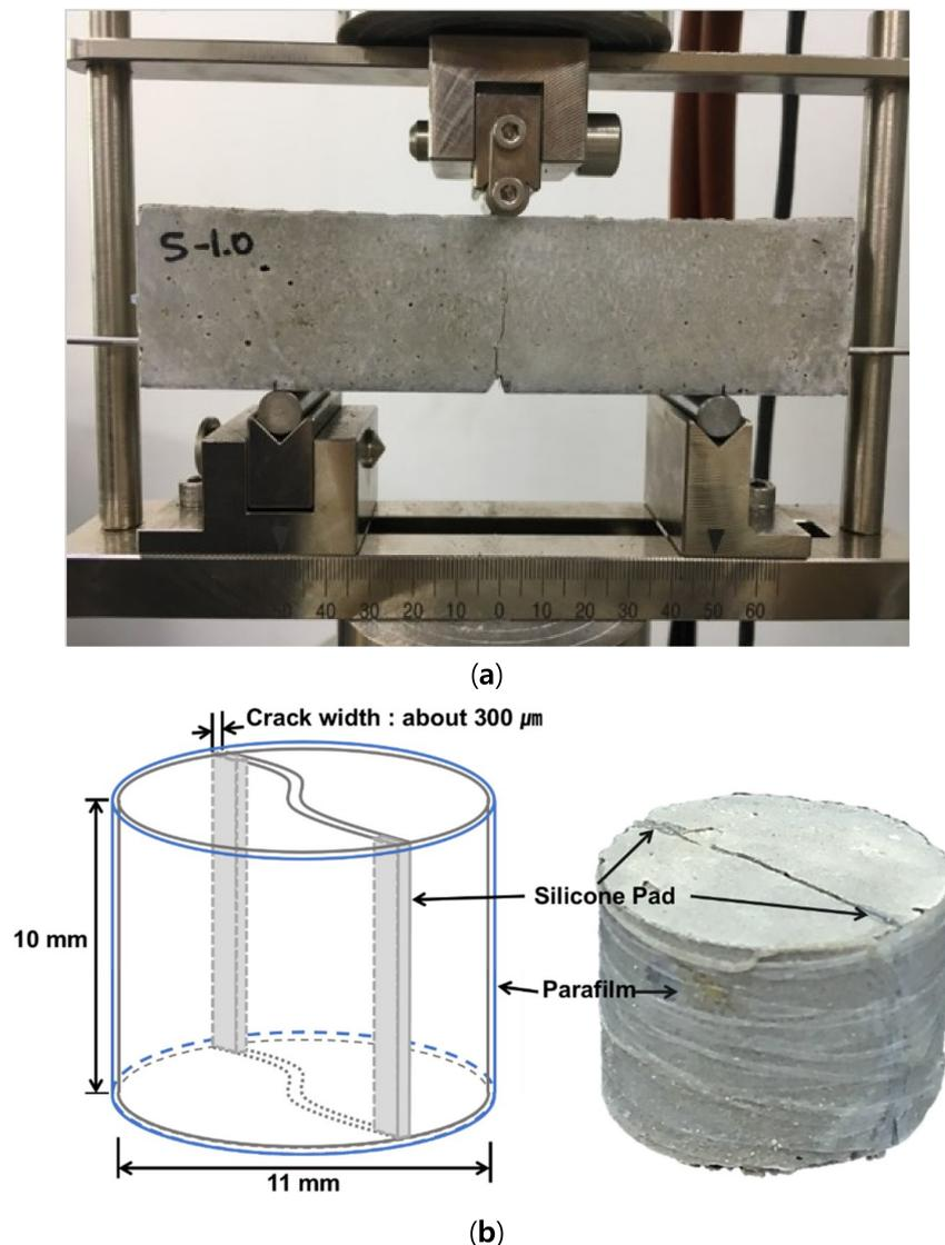
**Figure 2.** (a) Flexural crack-containing specimen for capillary water absorption test; (b) cracked specimen for X-ray micro-computed tomography (CT) analysis.
