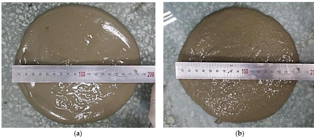
**Figure 1.** Flow measurement of (a) reference specimen (REF) and (b) superabsorbent polymers (SAPs)-added mixture.
