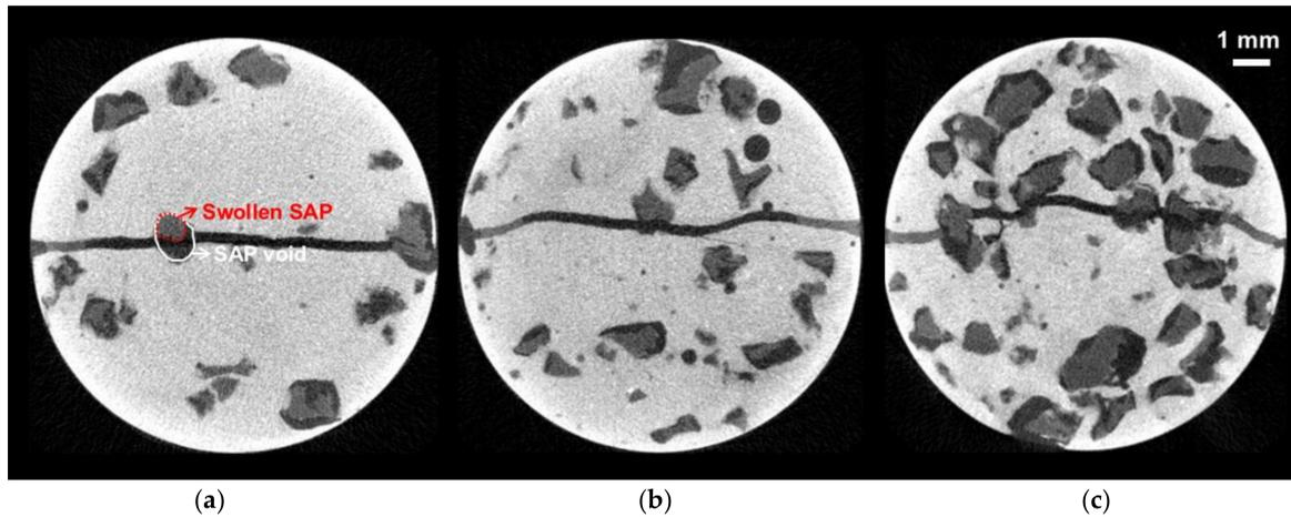
**Figure 8.** Gray-level X-ray micro CT image of (a) S-0.5, (b) S-1.0 and (c) S-1.5 specimen, taken after cracking.
