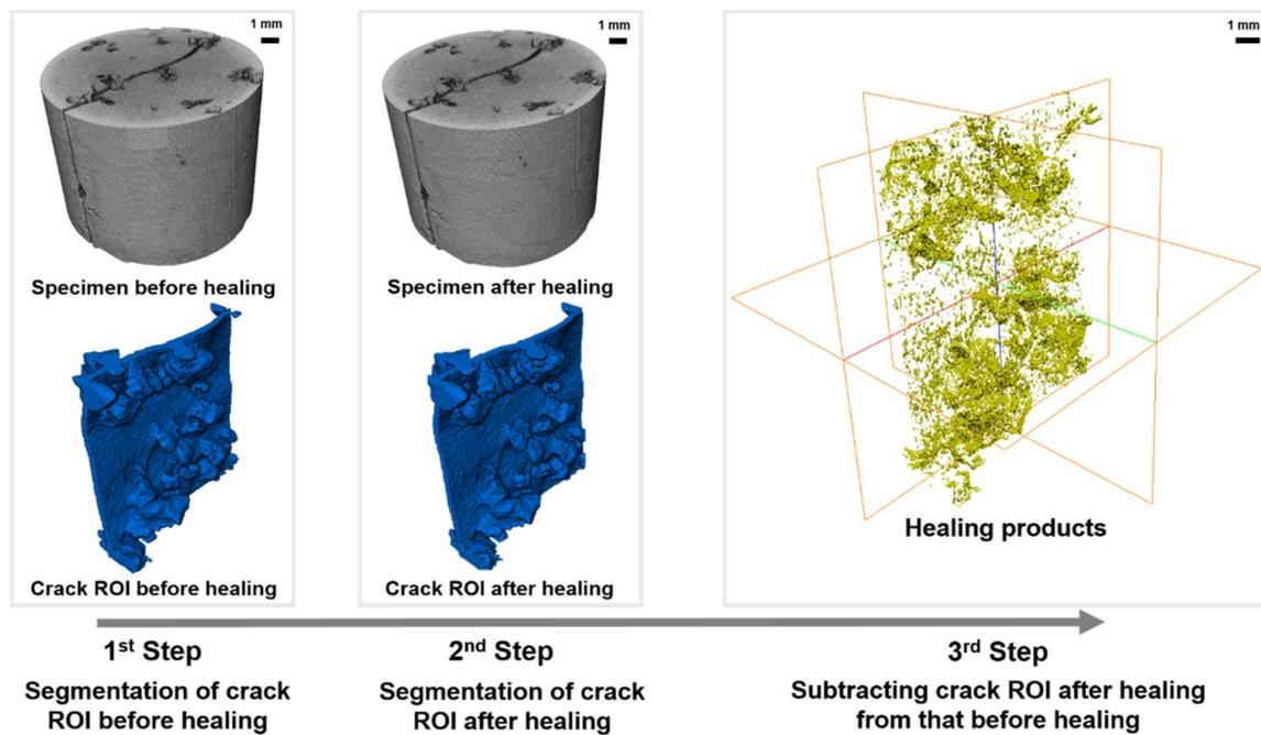
Figure 11. Segmentation of healing products in the crack ROI.
