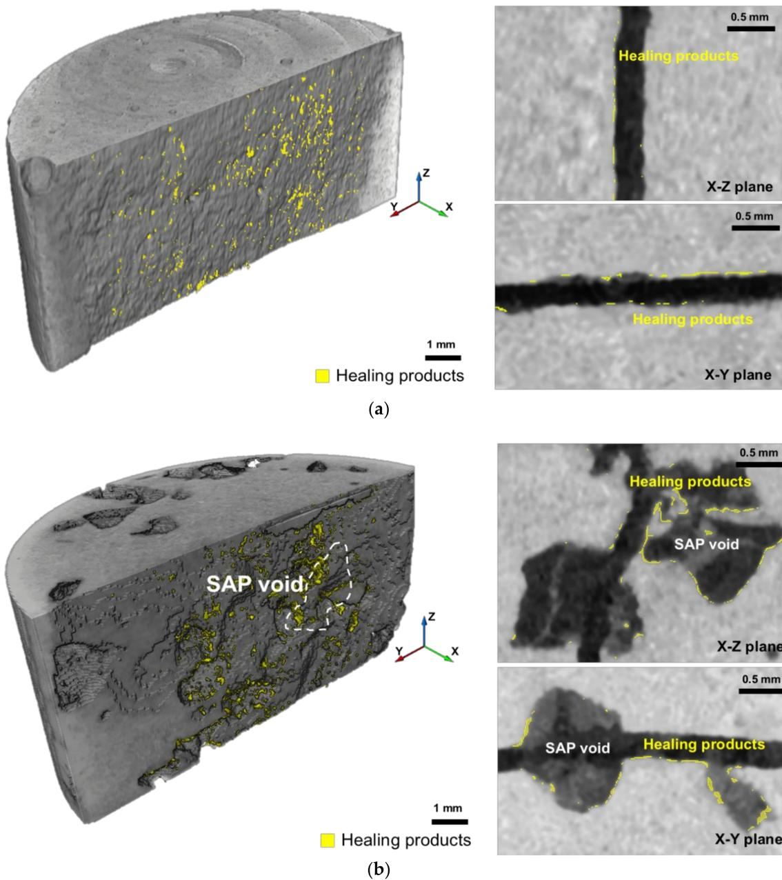
**Figure 12.** Three-dimensional images of healing products in the (a) reference specimen (REF) and (b) S-0.5 specimens after eight cycles, and cross-sectional images of the crack and SAP voids in X–Z and X–Y planes.
