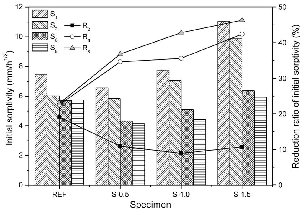
Figure 6. Initial sorptivity and reduction ratios of specimens exposed to wet/dry cycling.
