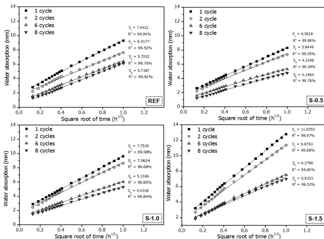
Figure 5. Water absorption of specimens over the square root of time, for different numbers of cycles.
