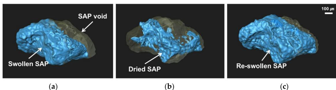
**Figure 9.** Three-dimensional images of SAP particles and voids in a crack surface of an S-0.5 specimen: (a) after cracking; (b) after a drying cycle; (c) after a wetting cycle.
