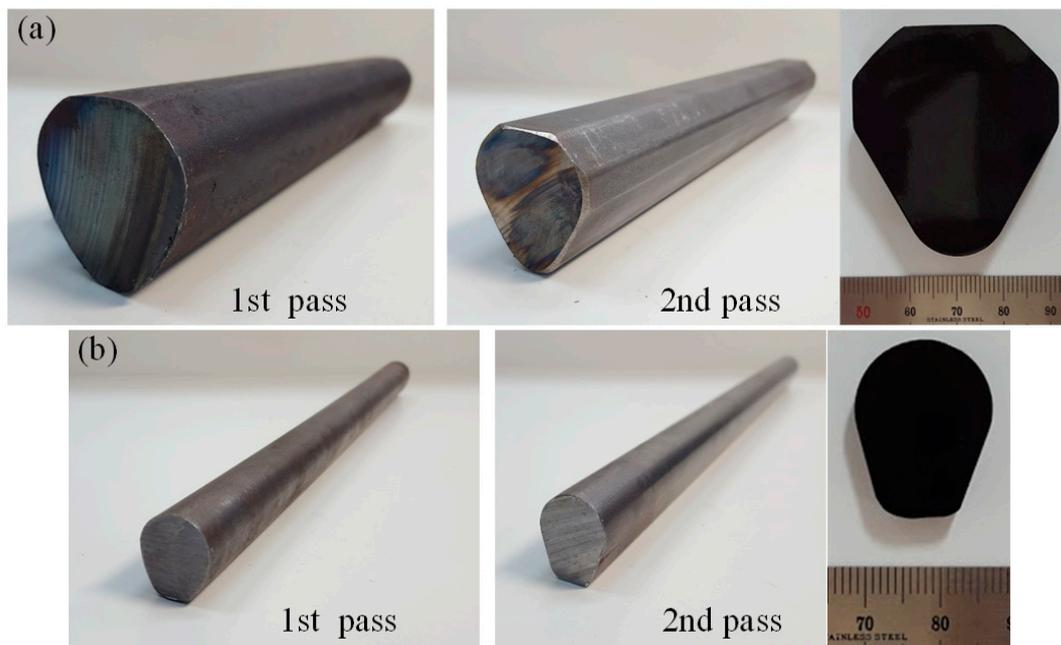
**Figure 21.** Drawn final products. (a) Diamond cross-section; (b) teardrop cross-section.
