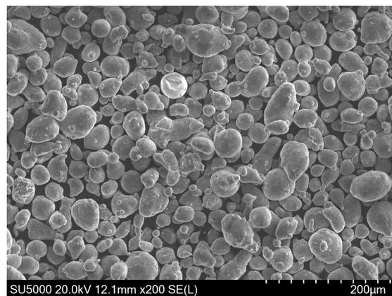
**Figure 4.** SEM of AlSi10Mg powders.
