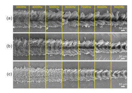
**Figure 11.** SEM image of the strip microstructure on Al alloy surface prepared by different laser beam pulse frequency: (**a**) 0.1 m/s; (**b**) 0.20 m/s; (**c**) 0.4 m/s.
