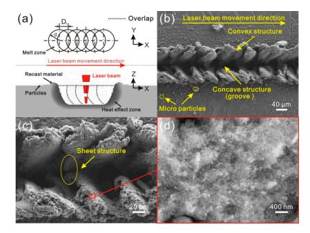
**Figure 5.** (a) Schematic of overlap degree of molten pools (multiple overlap of each melting zone, i.e.,  $0 < D_1 < d/2$ ); (b) SEM image of the microstructure on Al alloy surface (laser beam pulse frequency of 6000 Hz, laser beam scanning speed of 0.15 m/s); (c,d) high-magnification SEM image of the Al alloy surface.
