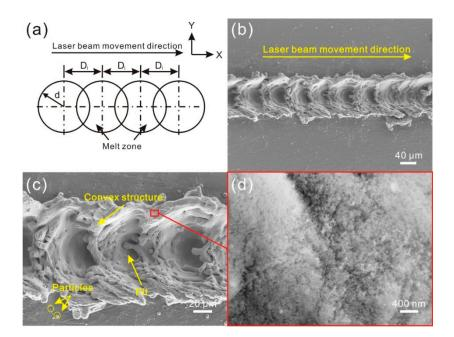
**Figure 4.** (a) Schematic of overlap degree of molten pools (overlap of each melting zone, i.e.,  $d \le D_1 < 2d$ ); (b) SEM image of the microstructure on alloy surface (laser beam pulse frequency of 8000 Hz, laser beam scanning speed of 0.4 m/s); (c,d) high-magnification SEM image of the microstructure.
