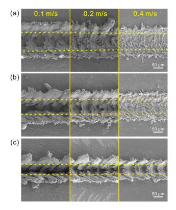
**Figure 10.** SEM image of the strip microstructure prepared by different laser beam scanning speed: (a) 3000 Hz; (b) 5000 Hz; (c) 8000 Hz.
