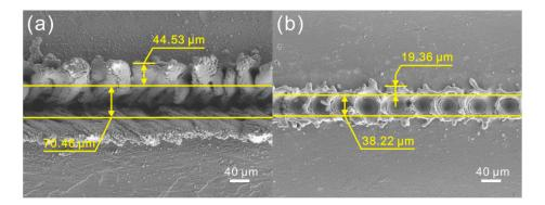
**Figure 14.** SEM images of the microstructure on Al alloy surface treated by laser micro-engraving: (**a**) laser beam pulse frequency of 5000 Hz, laser beam scanning speed of 0.05 m/s; (**b**) laser beam pulse frequency of 10,000 Hz, laser beam scanning speed of 0.4 m/s.
