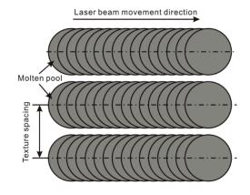
Figure 9. Schematic of overlap degree of melting zone.
