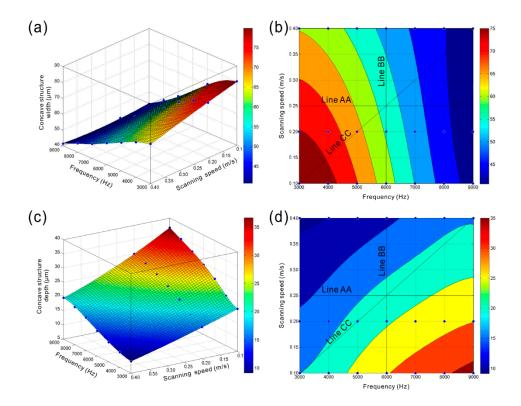
**Figure 12.** (**a**,**b**) Variations of concave structure width of the strip microstructure with laser beam pulse frequency and scanning speed; (**c**,**d**) Variations of depth of concave structure of the strip microstructure with laser beam pulse frequency and scanning speed.
