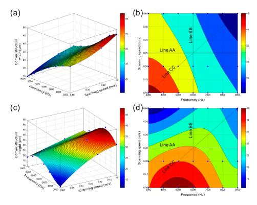
**Figure 13.** (**a**,**b**) Variations of convex structure width of the strip microstructure with laser beam pulse frequency and scanning speed; (**c**,**d**) Variations of convex structure height of the strip microstructure with laser beam pulse frequency and scanning speed.
