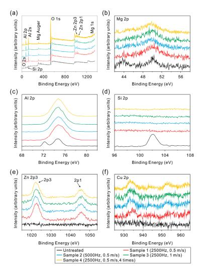
**Figure 15.** XPS spectra of the microstructure surface prepared by laser micro-engraving: (**a**) survey; (**b**) Mg 2p; (**c**) Al 2p; (**d**) Si 2p; (**e**) Zn 2p3; (**f**) Cu 2p.
