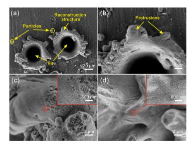
**Figure 2.** (a) SEM image of the microstructure on Al alloy surface treated by laser micro-engraving (laser beam pulse frequency of 10,000 Hz, laser beam scanning speed of 0 m/s); (b) high-magnification SEM image of the microstructure; (c) high-magnification SEM images of convex structure of the microstructure; (d) high-magnification SEM images of the pit.
