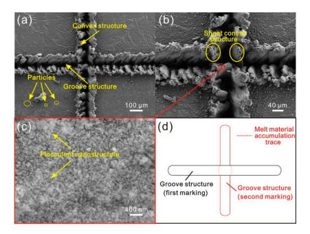
**Figure 6.** (a) SEM image of cross microstructure on Al alloy surface (laser beam pulse frequency of 6000 Hz, laser beam scanning speed of 0.15 m/s); (b,c) high-magnification SEM image of the microstructure; (d) schematic of the preparation process of cross structure.
