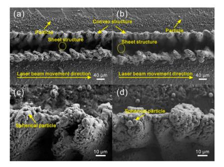
**Figure 7.** SEM image of the microstructure on Al alloy surface (laser beam pulse frequency of 6000 Hz, laser beam scanning speed of 0.15 m/s): (a) 2 times; (b) 4 times; (c,d) corresponding high-magnification SEM images.
