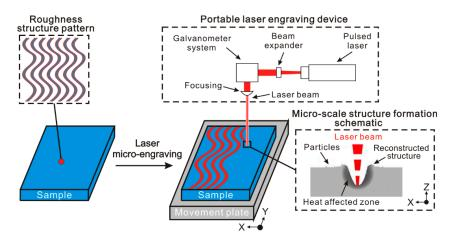
**Figure 1.** The treatment process and schematic of the micro-scale roughness structure construction approach (laser micro-engraving).
