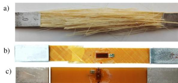
**Figure 3.** Failure forms of samples made of TVR 380 M12/26%/R-glass glass/epoxy material with layers orientation: (a)  $[0^\circ]_8$ , (b)  $[45^\circ / -45^\circ]_4$ , (c)  $[90^\circ]_8$ .
