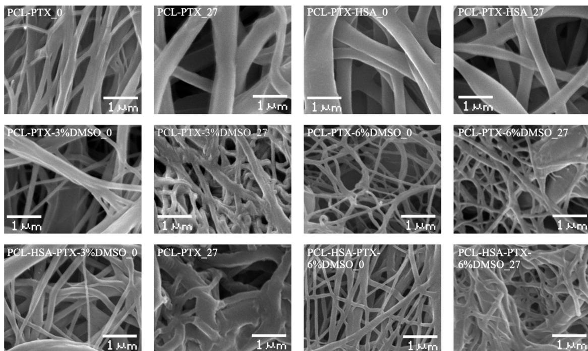
**Figure 1.** Microstructure of 3D matrices (SEM,  $\times 3000$  magnification). The digit following the matrix composition indicates the incubation time of the matrices in PBS.
