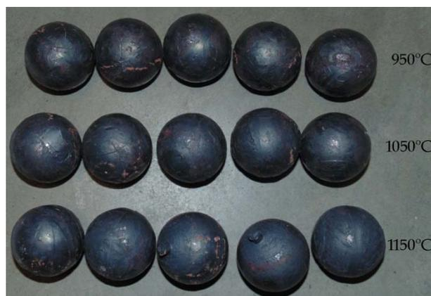
**Figure 5.** Shape of balls formed from 40 mm-diameter billet of varying initial temperatures.
