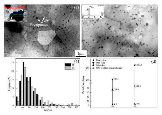
**Figure 1.** (**a**,**b**) STEM images showing the microstructure of the as-received #1 and #2 N36 Zr alloys, respectively; (**c**) the frequencies of particle lengths; (**d**) statistical results of the particle sizes.
