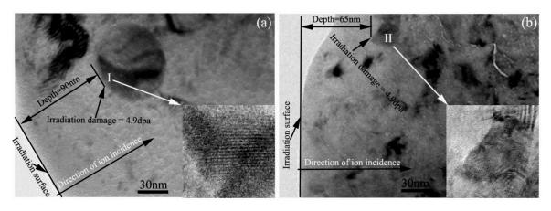
**Figure 5.** TEM bright field images showing the microstructure of the Zr alloys irradiated with  $1.43 \times 10^{15} \text{ Kr}^+/\text{cm}^2$  fluence at 360 °C. (a) Zr alloy #1; (b) Zr alloy #2.
