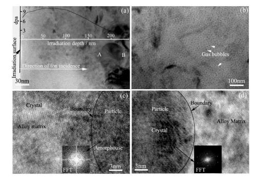
**Figure 4.** TEM bright field images showing the microstructure of Zr alloy #2 irradiated with  $2.86 \times 10^{15} \text{ Kr}^+/\text{cm}^2$  fluence at 320 °C. (a) Low magnification of an under-focused TEM image; (b) Over-focused TEM image showing gas bubbles; (c,d) HRTEM images showing the boundary area between a particle and the Zr matrix.
