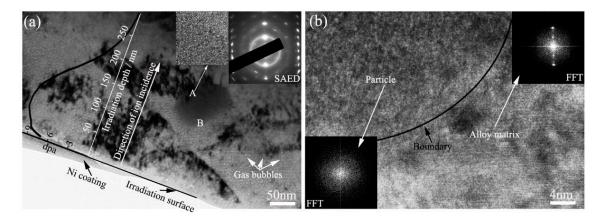
**Figure 3.** TEM bright field images showing the microstructure of Zr alloy #1 irradiated with  $2.86 \times 10^{15} \text{ Kr}^+/\text{cm}^2$  fluence at 320 °C. (a) Under-focused bright field image; (b) High-resolution TEM (HRTEM) image showing the boundary area between a particle and the Zr alloy matrix.
