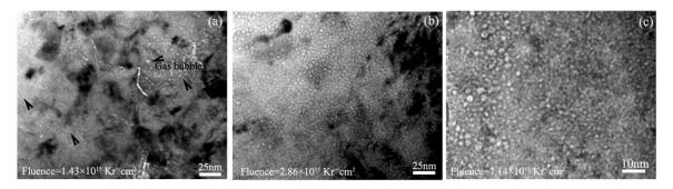
**Figure 6.** TEM bright field images showing the morphologies of Zr alloy #2 irradiated with (a)  $1.43 \times 10^{15}$ , (b)  $2.86 \times 10^{15}$ , and (c)  $7.14 \times 10^{15}$  Kr<sup>+</sup>/cm<sup>2</sup> fluence at 360 °C.
