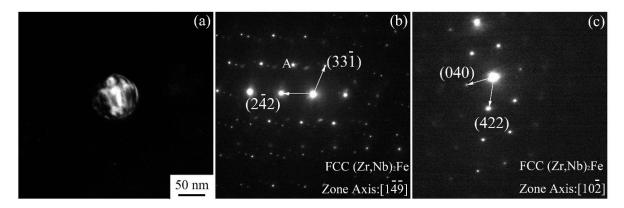
**Figure 2.** TEM dark field image and corresponding selected area electron diffraction patterns of a particle in Zr alloy #2. (a) TEM dark field image from the 'A' spot of the SAED (selected area electron diffraction) pattern in (b); (b,c) SAED patterns from different crystal zone axes.
