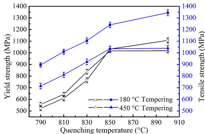
**Figure 3.** Yield strength and tensile strength as a function of quenching temperature tempered at 180 °C and 450 °C, respectively.
