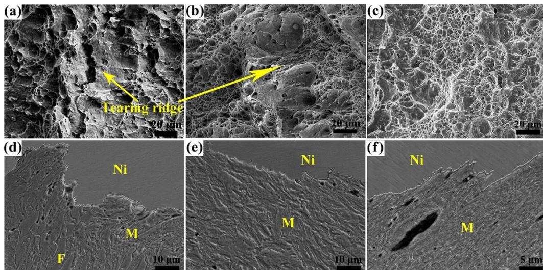
**Figure 11.** SEM images of the  $-40$  °C impact fracture morphology and microstructure underneath the fracture surface of the specimens tempered at 450 °C with ferrite content of (a,d) 37 vol%, (b,e) 3 vol%, and (c,f) none, respectively.
