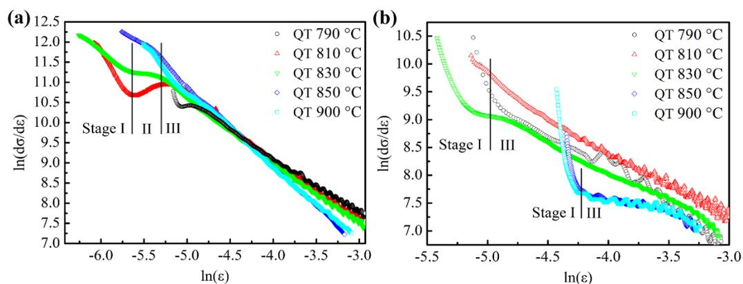
**Figure 8.**  $D_{C-J}$  plots of  $\ln(d\sigma/d\varepsilon)$  versus  $\ln(\varepsilon)$  for specimens quenched from different temperatures and tempered at (a) 180 °C and (b) 450 °C, respectively.
