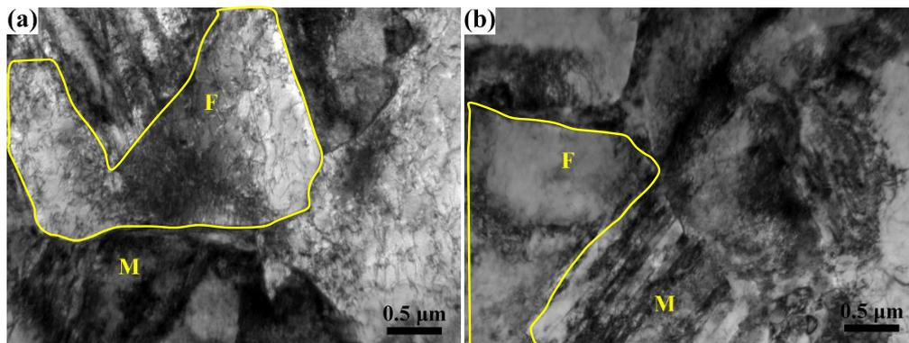
**Figure 4.** Representative TEM microstructures of specimens with ferrite and martensite quenched from 810 °C and tempered at (a) 180 °C and (b) 450 °C, respectively.
