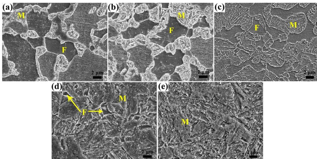
**Figure 2.** SEM microstructure of HSLA steel quenched from (a) 790 °C, (b) 810 °C, (c) 830 °C, (d) 850 °C, and (e) 900 °C, and tempered at 450 °C.
