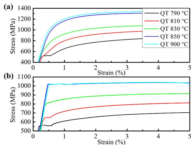
**Figure 5.** Yielding stage of stress–strain curves of specimens quenched from different temperatures and tempered at (a) 180 °C and (b) 450 °C, respectively (QT = quenching temperature).
