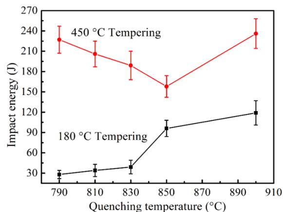
**Figure 9.**  $-40$  °C Charpy V-notched impact energy versus quenching temperature of the specimens tempered at  $180$  °C and  $450$  °C, respectively.
