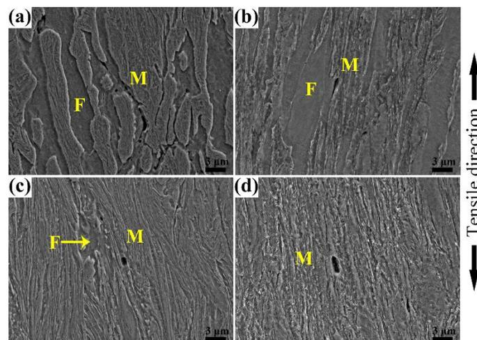
**Figure 7.** SEM microstructure of deformed HSLA steel next to the tensile fracture surface. (a,b) with 37 vol% ferrite tempered at 180 °C and 450 °C, respectively, and (c,d) with 3 vol% ferrite tempered at 180 °C and 450 °C, respectively.
