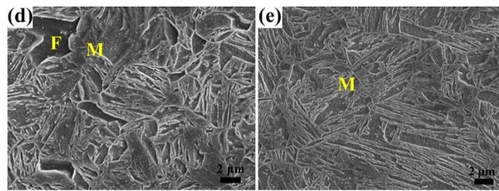
**Figure 1.** SEM microstructure of high-strength low-alloy (HSLA) steel quenched from (a) 790 °C, (b) 810 °C, (c) 830 °C, (d) 850 °C, and (e) 900 °C, and tempered at 180 °C. (F = ferrite and M = martensite).
