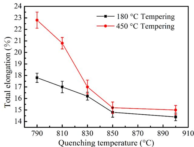
**Figure 6.** Total elongation as a function of quenching temperature tempered at 180 °C and 450 °C, respectively.
