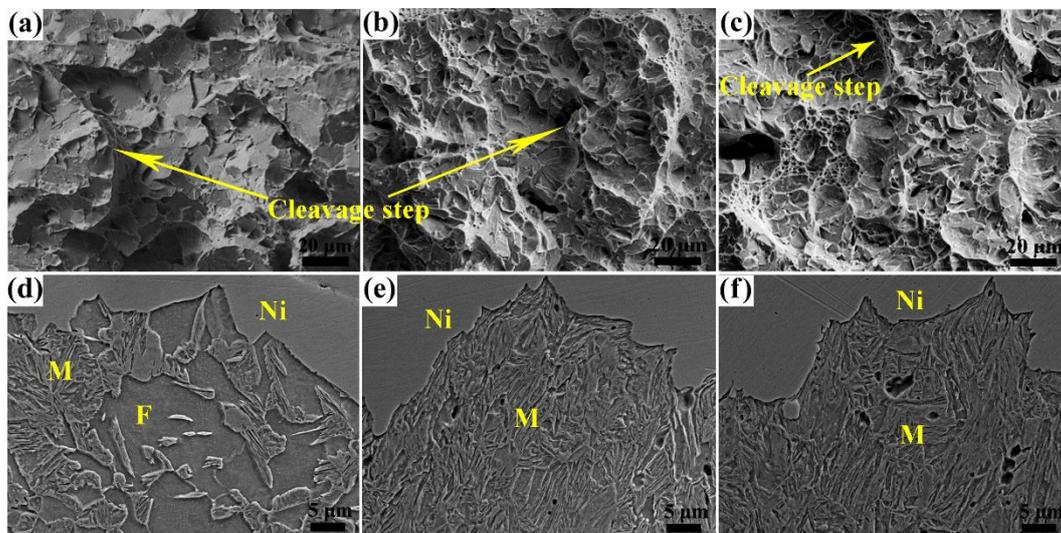
**Figure 10.** SEM images of the  $-40$  °C impact fracture morphology and microstructure underneath the fracture surface of the specimens tempered at  $180$  °C with ferrite content of (a,d) 37 vol%, (b,e) 3 vol%, and (c,f) none, respectively. (Ni = coated nickel layer).
