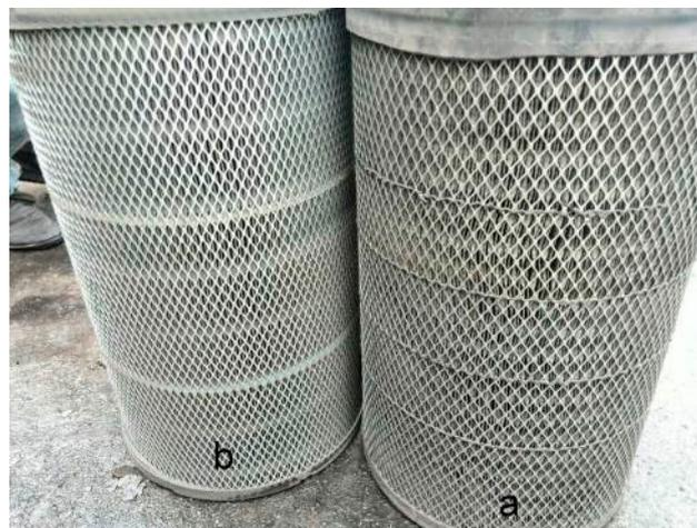
**Figure 5.** OEM inlet air filter (a) and new submicro-fiber filter (b).
