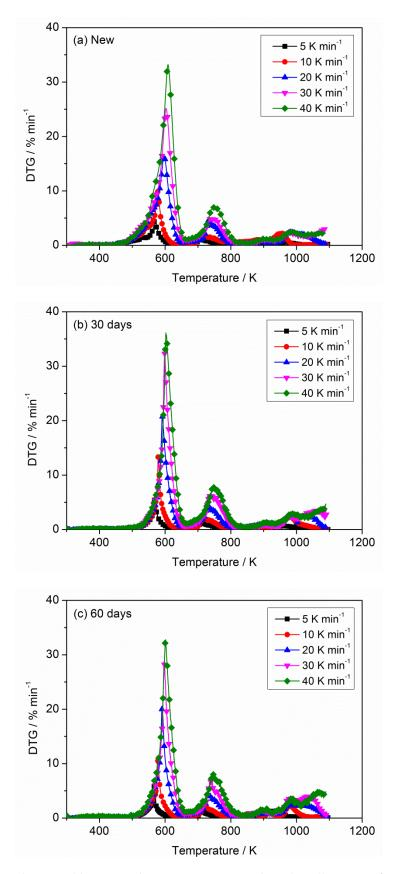
**Figure 3.** Mass loss rate (derivative thermogravimetric analysis (DTG)) curves of PVC sheath at different heating rates in nitrogen atmosphere: (**a**) new; (**b**) aged 30 days and (**c**) aged 60 days.
