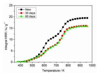
Figure 8. Integral HRR (total heat release (THR)) of PVC sheaths for new and aged cables.
