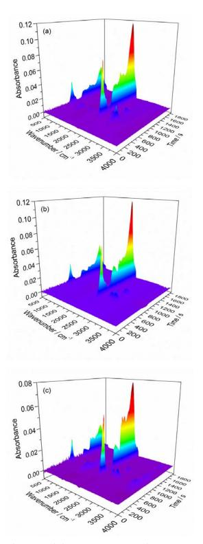
**Figure 6.** Typical three-dimensional thermogravimetric analysis-Fourier transform infrared (3D TG-FTIR) spectrogram of PVC sheath at a heating rate of 30 K min<sup>-1</sup>: (a) new; (b) aged 30 days; and, (c) aged 60 days.
