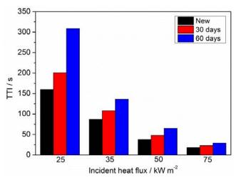
**Figure 9.** Time to ignition (TTI) of PVC sheaths for new and aged cables with different incident heat fluxes.
