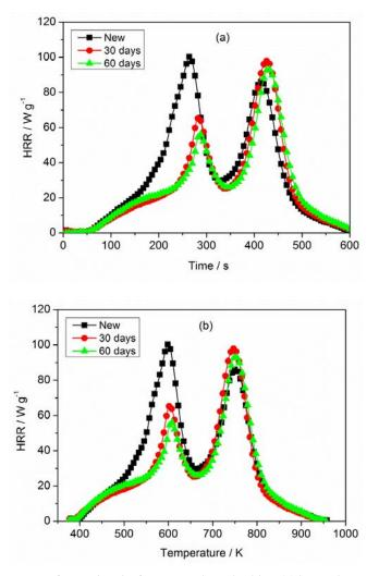
**Figure 7.** Heat release rate of PVC sheaths for new and aged cables: (**a**) heat release rate (HRR) vs. time and (**b**) HRR vs. temperature.
