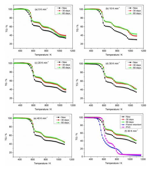
**Figure 4.** Comparison of TG of PVC sheaths for new and aged cables at different heating rates in nitrogen atmosphere. (**a**) 5 K min<sup>-1</sup>; (**b**) 10 K min<sup>-1</sup>; (**c**) 20 K min<sup>-1</sup>; (**d**) 30 K min<sup>-1</sup>; (**e**) 40 K min<sup>-1</sup> and (**f**) 30 K min<sup>-1</sup> involving raw materials.
