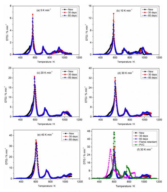
**Figure 5.** Comparison of DTG of PVC sheaths for new and aged cables at different heating rates in nitrogen atmosphere. (**a**)  $5 \text{ K min}^{-1}$ ; (**b**)  $10 \text{ K min}^{-1}$ ; (**c**)  $20 \text{ K min}^{-1}$ ; (**d**)  $30 \text{ K min}^{-1}$ ; (**e**)  $40 \text{ K min}^{-1}$  and (**f**)  $30 \text{ K min}^{-1}$  involving raw materials.
