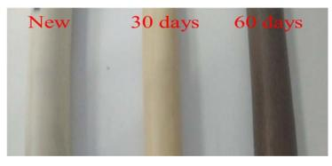
Figure 1. Digital photographs of polyvinyl chloride (PVC) sheaths before and after thermal aging.
