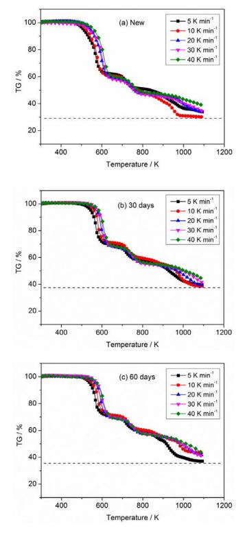
**Figure 2.** Mass loss (thermogravimetric analysis (TG)) curves of PVC sheaths at different heating rates in nitrogen atmosphere: (**a**) new; (**b**) aged 30 days and (**c**) aged 60 days.
