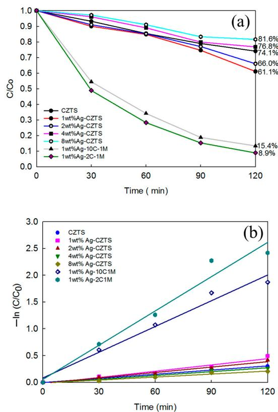
**Figure 8.** Photocatalytic activity under solar irradiation through the hybridized various weight percentages of AgNO<sub>3</sub> precursor: 1, 2, 4, and 8 wt% Ag/CZTS and the ratios of 10:1 and 2:1 of 1 wt% Ag/CZTS and 1T-2H MoS<sub>2</sub>; (a) the degradation of MB; and (b) the photocatalytic degradation kinetics evolution.
