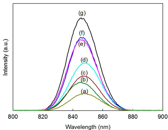
**Figure 6.** PL spectra of (a) 2:1 ratio of 1 wt% Ag/CZTS and 1T-2H MoS<sub>2</sub>; (b) 10:1 ratio of 1 wt% Ag/CZTS and 1T-2H MoS<sub>2</sub>; (c) 1 wt% Ag/CZTS; (d) 2 wt% Ag/CZTS; (e) CZTS; (f) 4 wt% Ag/CZTS; and (g) 8 wt% Ag/CZTS.
