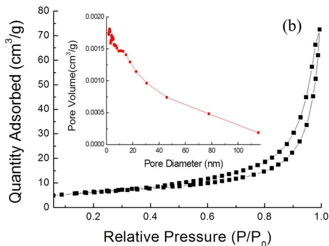
**Figure 4.** N<sub>2</sub> adsorption/desorption isotherms of (a) CZTS powders, and (b) 1T-2H MoS<sub>2</sub> microflower powders; insets are BJH pore size distribution plots, respectively.
