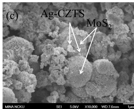
**Figure 2.** Scanning electron microscopy (SEM) images of the prepared CZTS powders with the (a) 1 wt% Ag doped on CZTS powder; (b) 1T-2H MoS<sub>2</sub> microflower; and (c) the 2:1 ratio of 1 wt% Ag/CZTS and 1T-2H MoS<sub>2</sub>.
