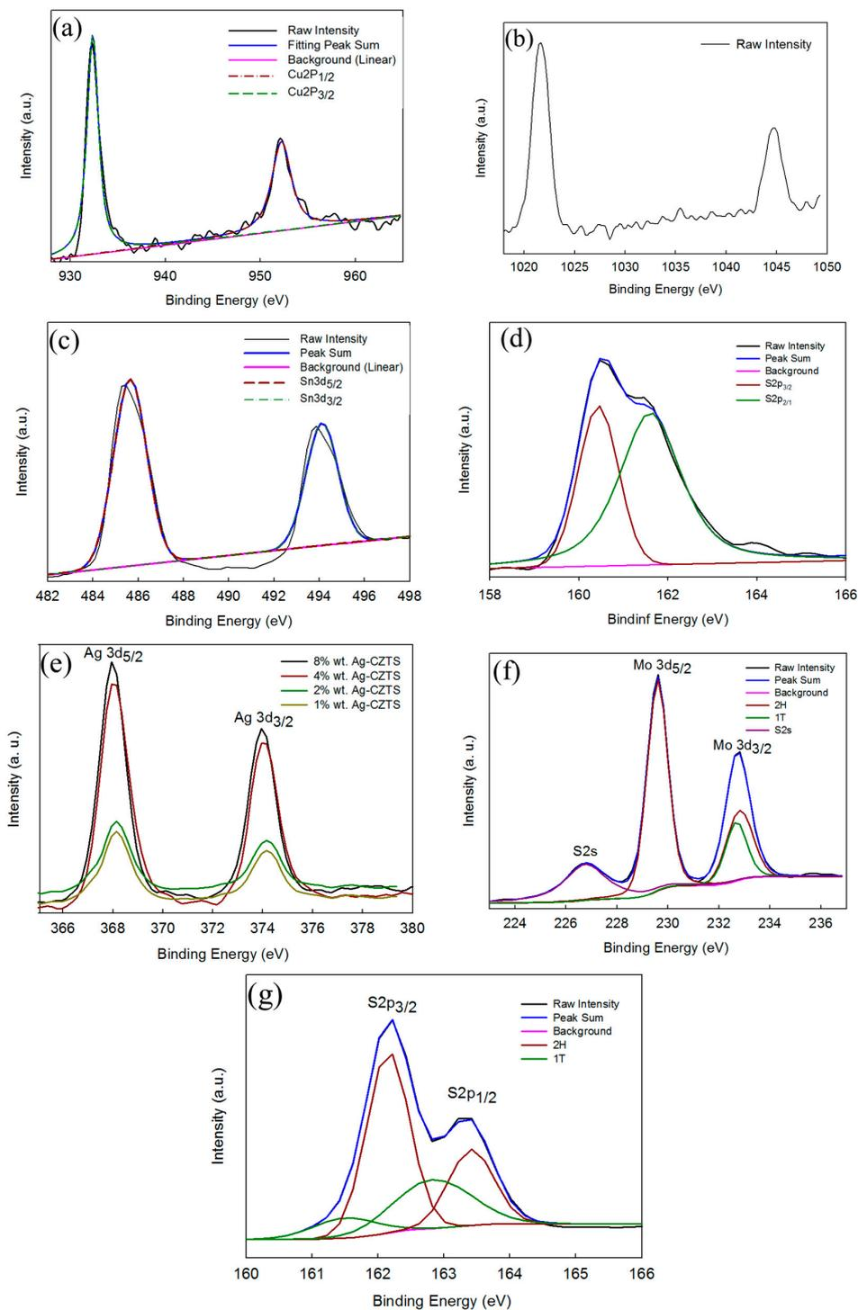
**Figure 7.** High-resolution XPS characterization of as-synthesized (a) Cu 2p; (b) Zn 2p; (c) Sn 3d; (d) S 2p; (e) Ag NPs; (f) Mo 3d; and (g) S 2p.
