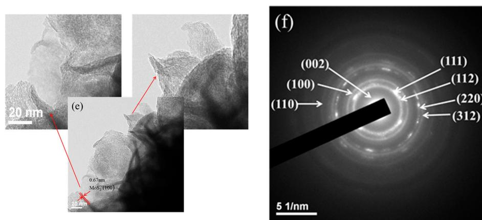
**Figure 3.** TEM images (a) 1 wt% Ag doped on CZTS powders; (b) 1T-2H MoS<sub>2</sub> microflower; (c) 2:1 ratio of 1 wt% Ag/CZTS and 1T-2H MoS<sub>2</sub>; HRTEM images of (d) 1 wt% Ag/CZTS; (e) 1T-2H MoS<sub>2</sub> microflower; and (f) SAED micrographs of 2:1 ratio of 1 wt% Ag/CZTS and 1T-2H MoS<sub>2</sub>.
