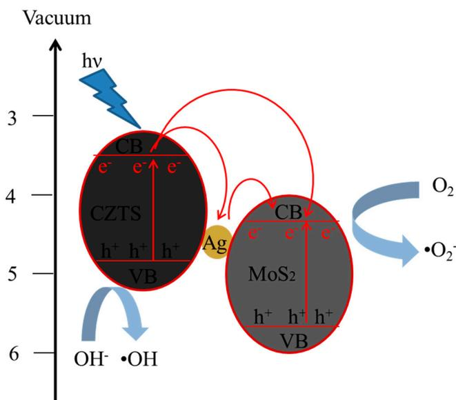
**Figure 9.** Schematic diagram for proposed photodegradation mechanism of methylene blue solution in the presence of the Ag/CZTS hybridized 1T-2H MoS<sub>2</sub> photocatalyst.
