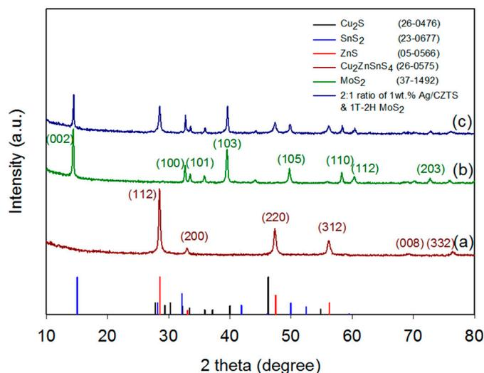
**Figure 1.** XRD pattern of (a) CZTS powders using the conventional hydrothermal process (CHT) at 180 °C for 72 h; (b) MoS<sub>2</sub> powder using the CHT process at 200 °C for 24 h; (c) 2:1 ratio of 1 wt% Ag/CZTS and 1T-2H MoS<sub>2</sub>.
