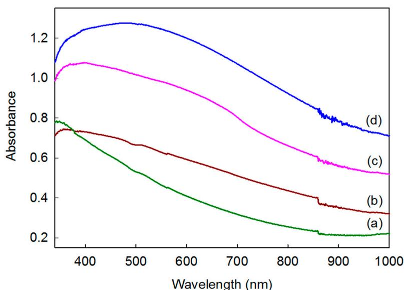
**Figure 5.** UV-VIS absorption spectra of (a) CZTS; (b) 1 wt% Ag/CZTS; (c) 10:1 ratio of 1 wt% Ag/CZTS and 1T-2H MoS<sub>2</sub>; and (d) 2:1 ratio of 1 wt% Ag/CZTS and 1T-2H MoS<sub>2</sub>.
