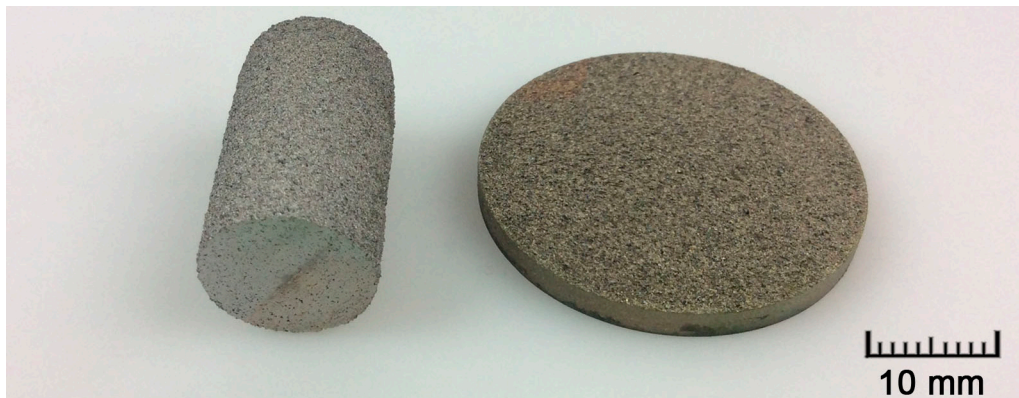
Figure S2. Prepared plasma-sprayed titanium: bulk sample and titanium layer on a Ti6Al4V plate.
