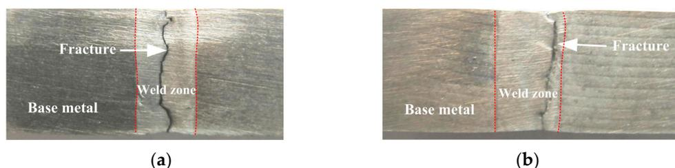
**Figure 14.** Fracture tensile samples of (a) autogenous laser welding; and (b) PCALW.
