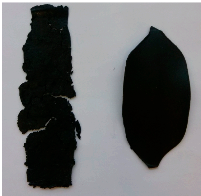
Figure 20. Materials MU2 (left) and MU3 (right) after pressing at same conditions.
