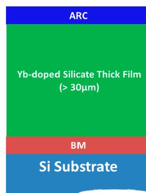
**Figure 14.** Schematic structure of the active disks prepared.
