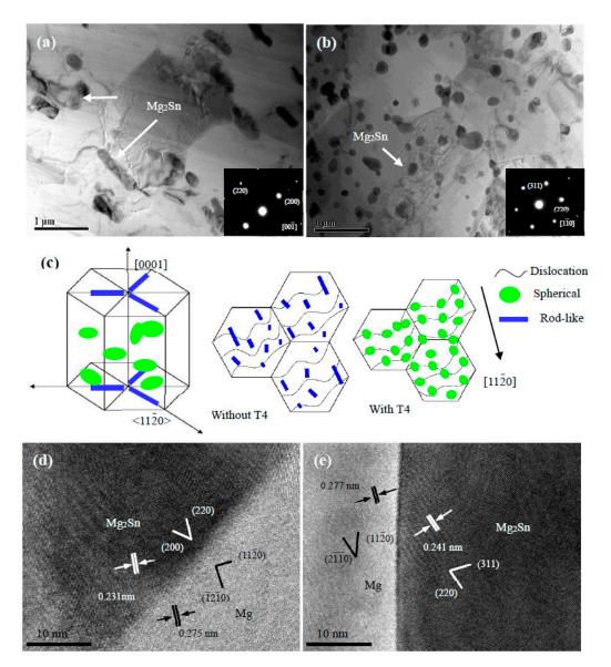
**Figure 4.** Bright field TEM images of DRXed region of extruded TZA822 alloys taken from the zone axis of [0001] (inset: SAED pattern) (**a**) without T4; (**b**) with T4; (**c**) The schematic illustration of the two different types of precipitates; (**d**,**e**) HR-TEM of rod-like and spherical precipitates.
