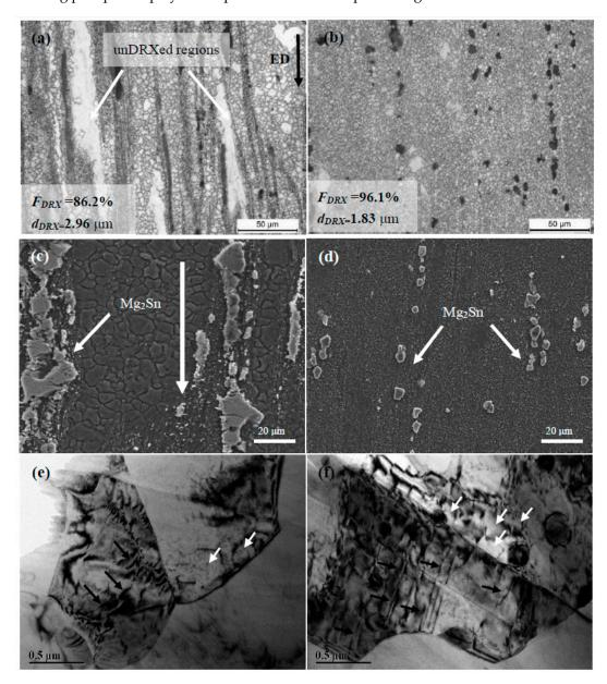
**Figure 2.** OM, SEM-SE and TEM images of extruded TZA822 alloys: (**a**,**c**,**e**) without T4 and (**b**,**d**,**f**) with T4, respectively.
