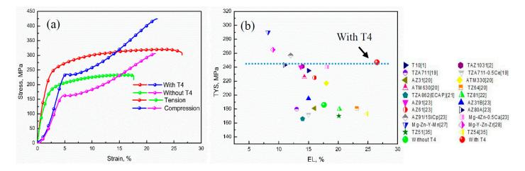
Figure 6. (a) Tensile and compressive stress-strain curves of the extruded TZA822 alloys; (b) TYS and EL of various Mg based wrought alloys.
