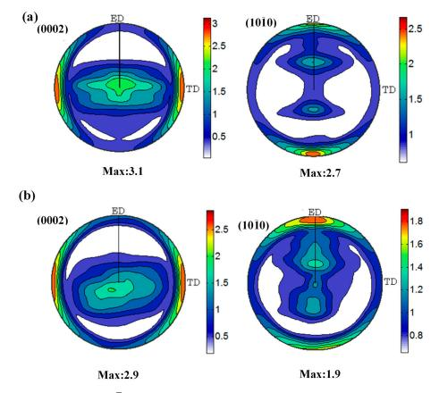
**Figure 5.** The (0002) and (1010) pole figures of extruded TZA822 alloys. (**a**) Without T4 and (**b**) with T4, respectively.
