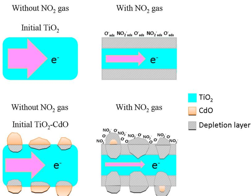
Figure 9. A schematic of gas sensing mechanisms for the TiO<sub>2</sub> and TiO<sub>2</sub>-CdO rods on exposure to NO<sub>2</sub> gas. The size of arrows represented the current degree in the TiO<sub>2</sub>.
