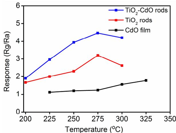
**Figure 6.** Gas sensing response value vs. operating temperature of the CdO film, TiO<sub>2</sub> rods, and TiO<sub>2</sub>-CdO rods.
