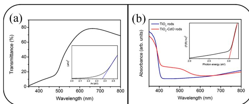
**Figure 4.** (a) Transmittance spectrum of the CdO film. The inset in (a) shows the Tauc plot of the CdO film. (b) Absorbance spectra of the TiO<sub>2</sub> and TiO<sub>2</sub>-CdO rods. The inset in (b) shows the bandgap of the TiO<sub>2</sub> rods is approximately 3.02 eV.
