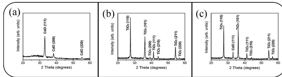
**Figure 2.** (a) XRD pattern of the CdO film. (b) XRD pattern of the TiO<sub>2</sub> rods. (c) XRD pattern of the TiO<sub>2</sub>-CdO rods.
