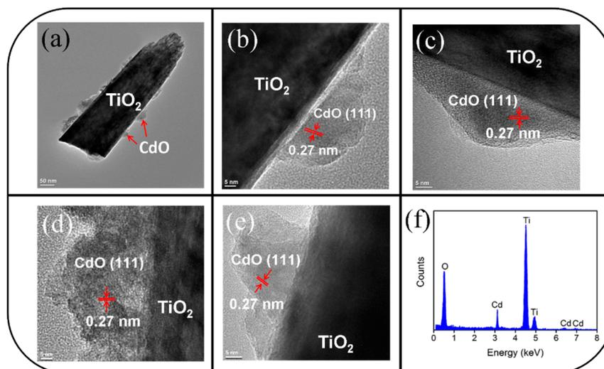
**Figure 3.** TEM analyses of the TiO<sub>2</sub>-CdO composite rod: (a) Low-magnification TEM image of the TiO<sub>2</sub>-CdO rod; (b–e) HRTEM images taken from the local regions of the rod; (f) EDS spectra of Ti, Cd, and O elements taken from the rod.
