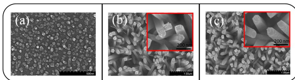
**Figure 1.** (a) SEM image of the CdO film. (b) SEM image of the  $TiO_2$  rods. (c) SEM image of the  $TiO_2$ -CdO rods.
