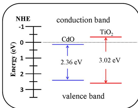
Figure 8. Energy diagram of the TiO<sub>2</sub> and CdO phases.
